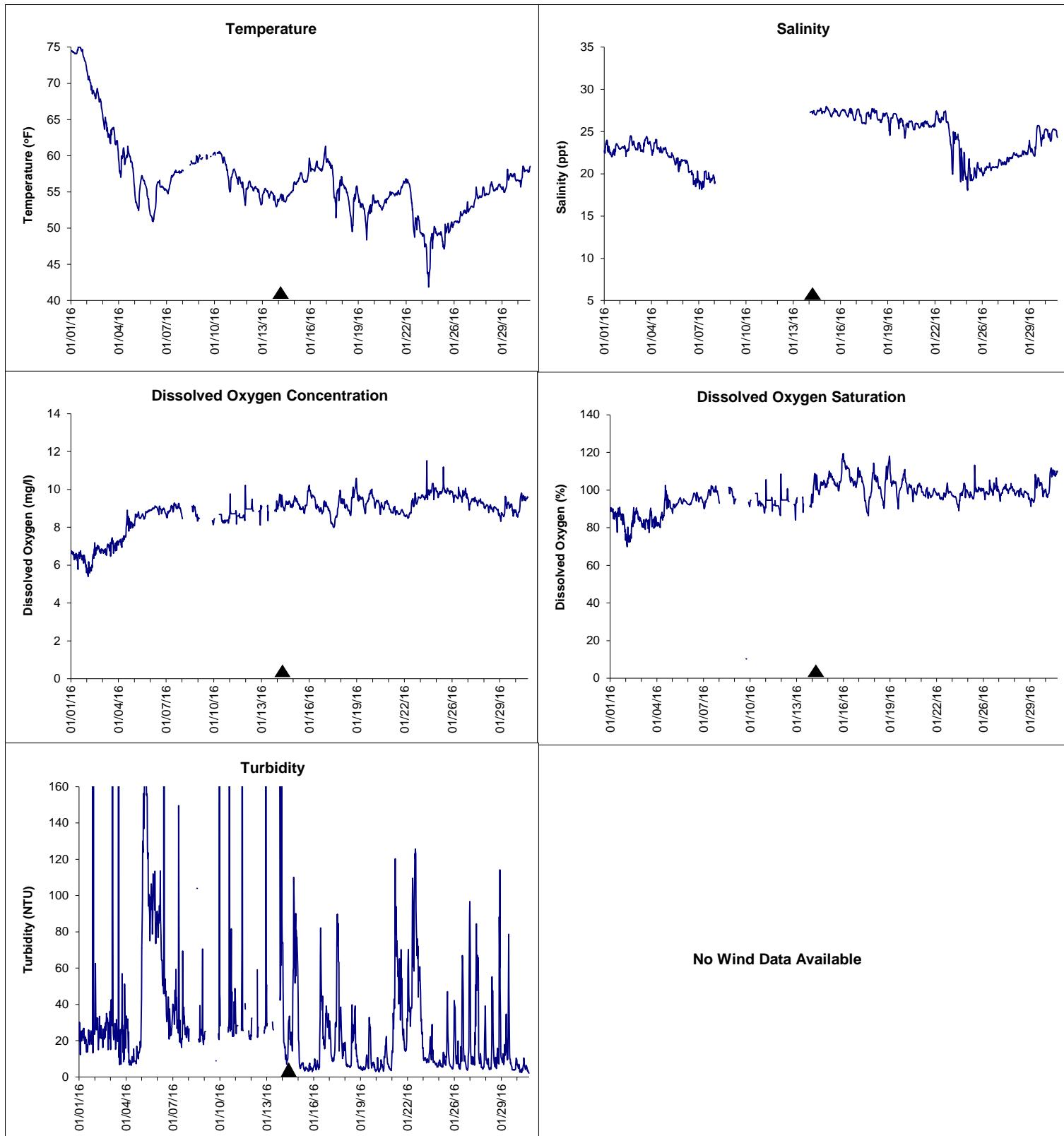
▲ Monitoring Equipment Exchanged (sonde deployment)
