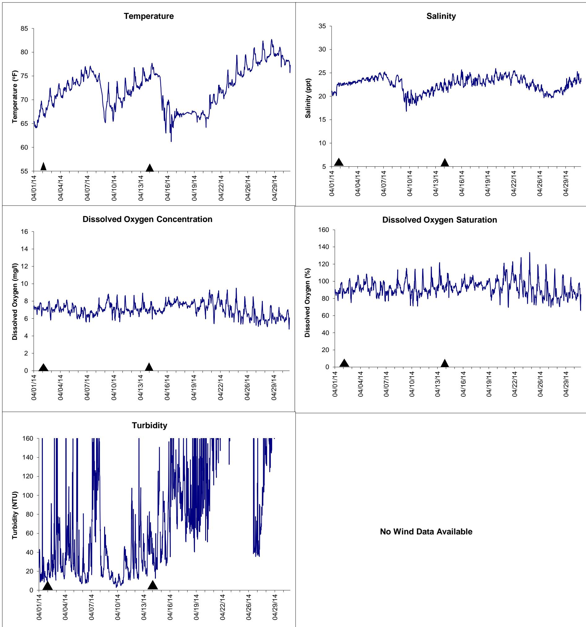
▲ Monitoring Equipment Exchanged (sonde deployment)
