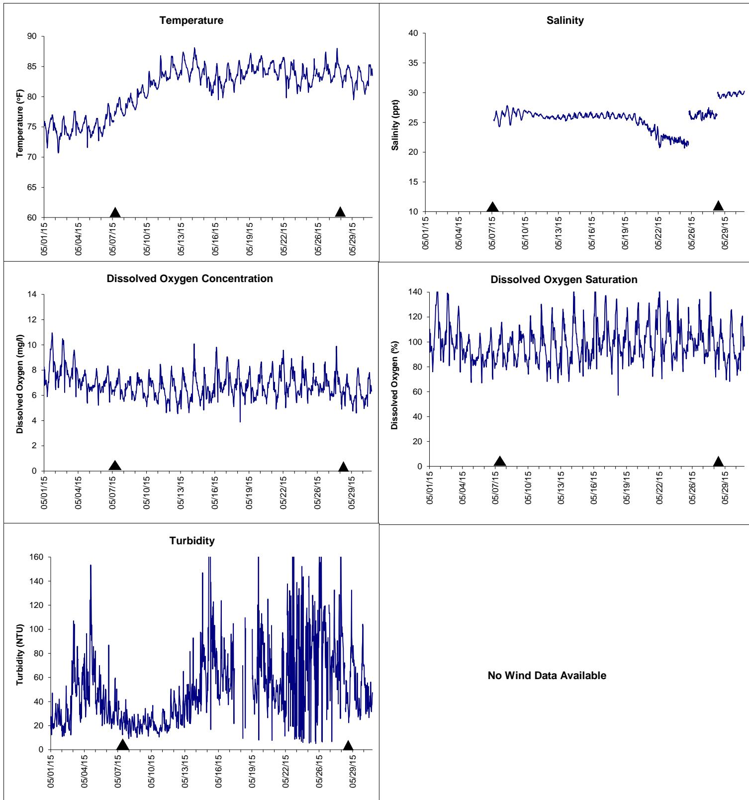
▲ Monitoring Equipment Exchanged (sonde deployment)
