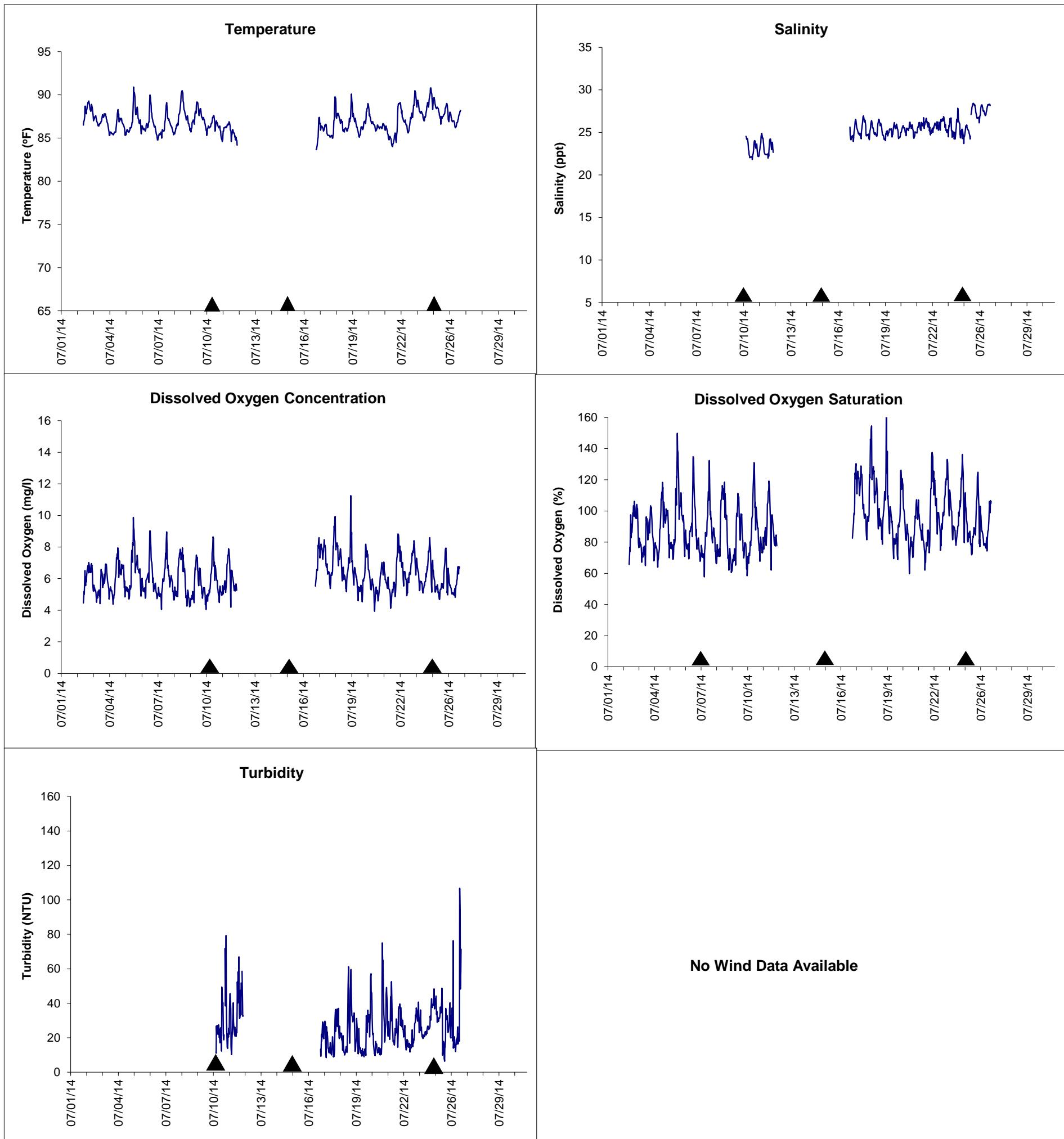
▲ Monitoring Equipment Exchanged (sonde deployment)
