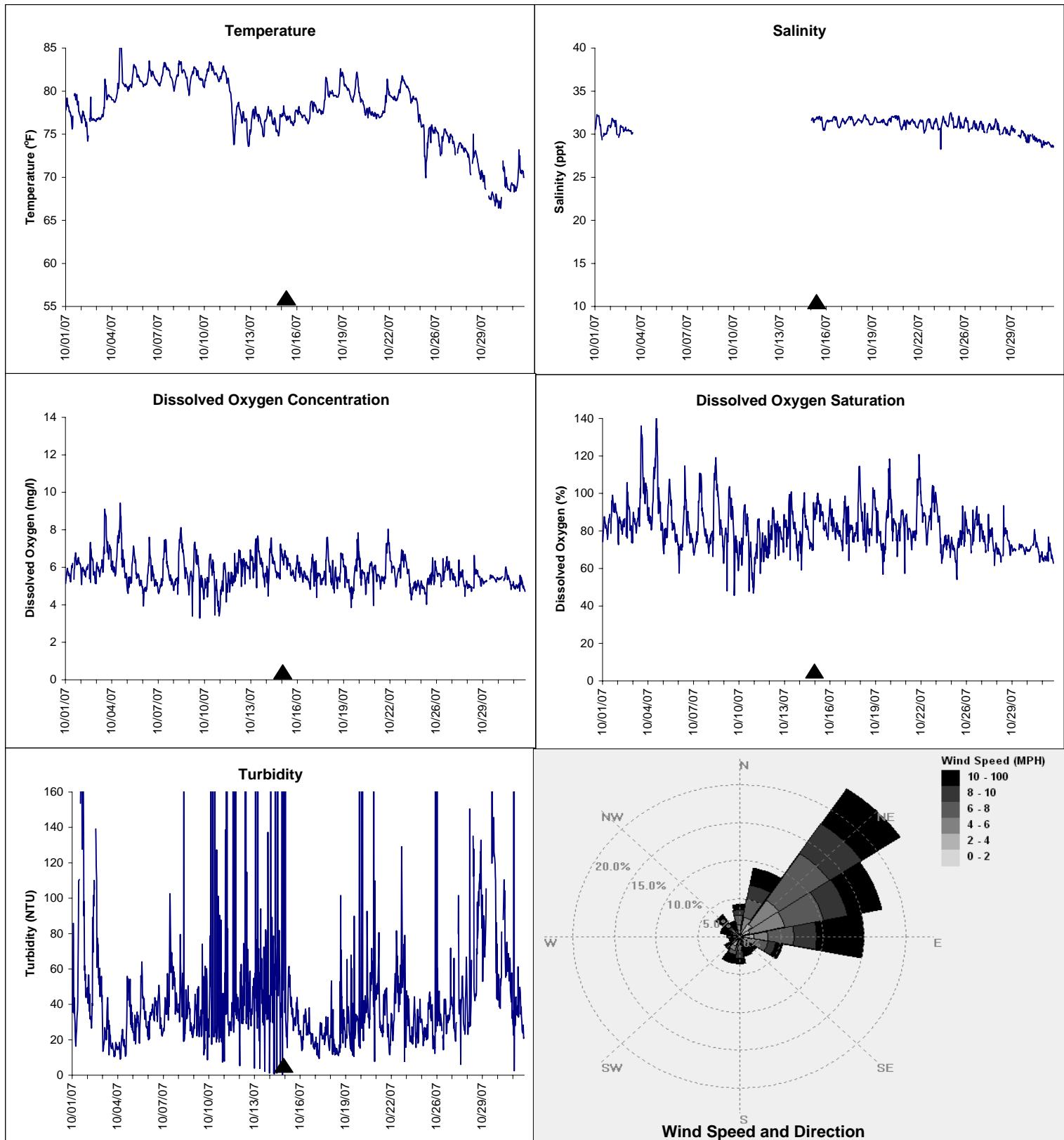
▲ Monitoring Equipment Exchanged (sonde deployment)
