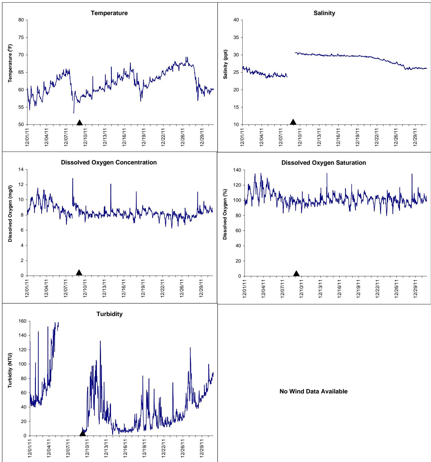
▲ Monitoring Equipment Exchanged (sonde deployment)
