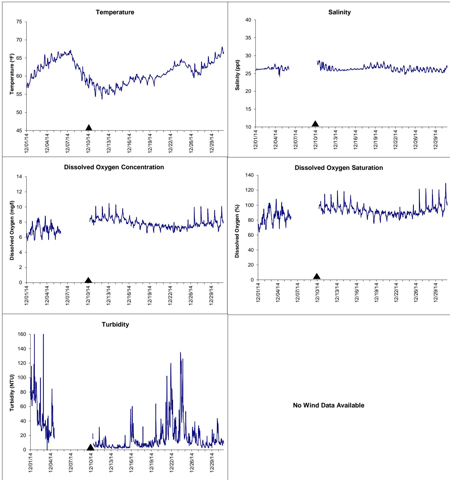
▲ Monitoring Equipment Exchanged (sonde deployment)
