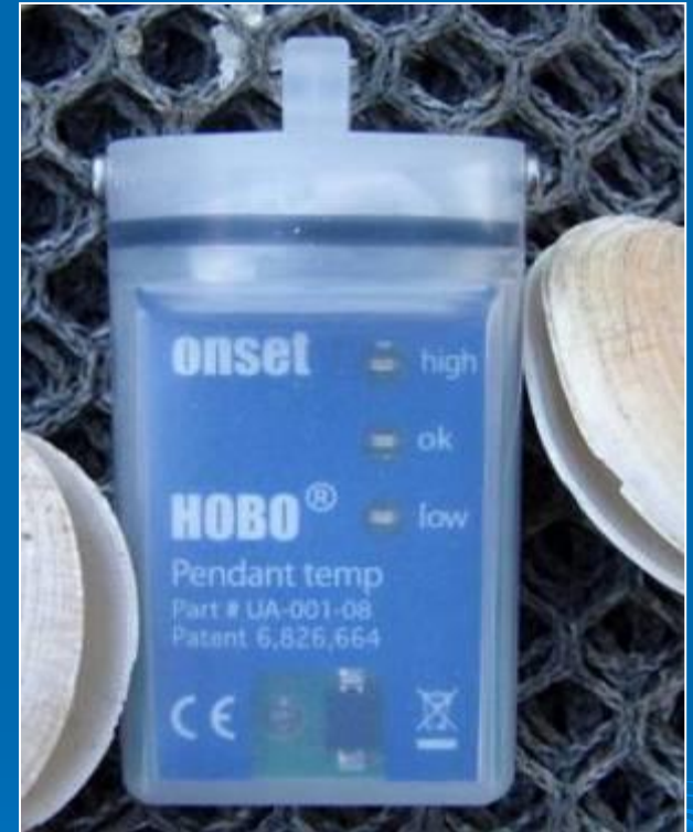
HOBOnset® Pendant Temperature Data Logger (2.3 x 1.3 x 0.9 inches)
