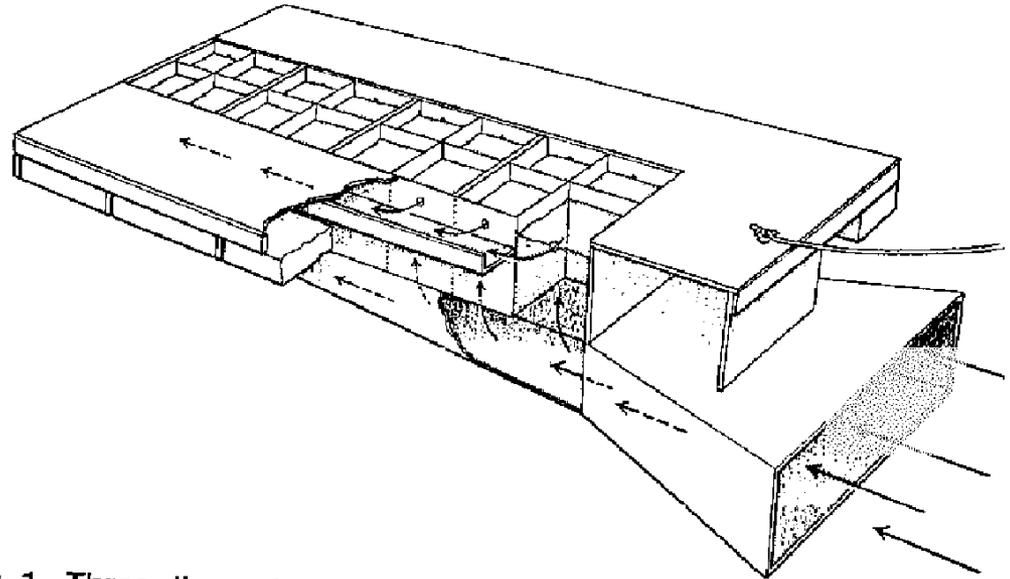
Fig. 1 - Three-dimensional schematic of the Tidal-Powered Upwelling Nursery System.
