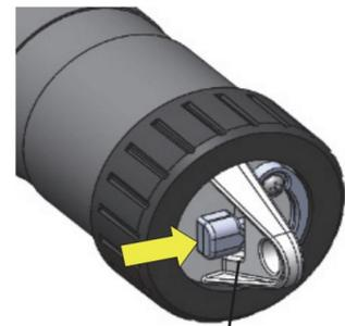
Push switch into the gap beneath the mounting lanyard to start or stop logging or to wake up the logger
