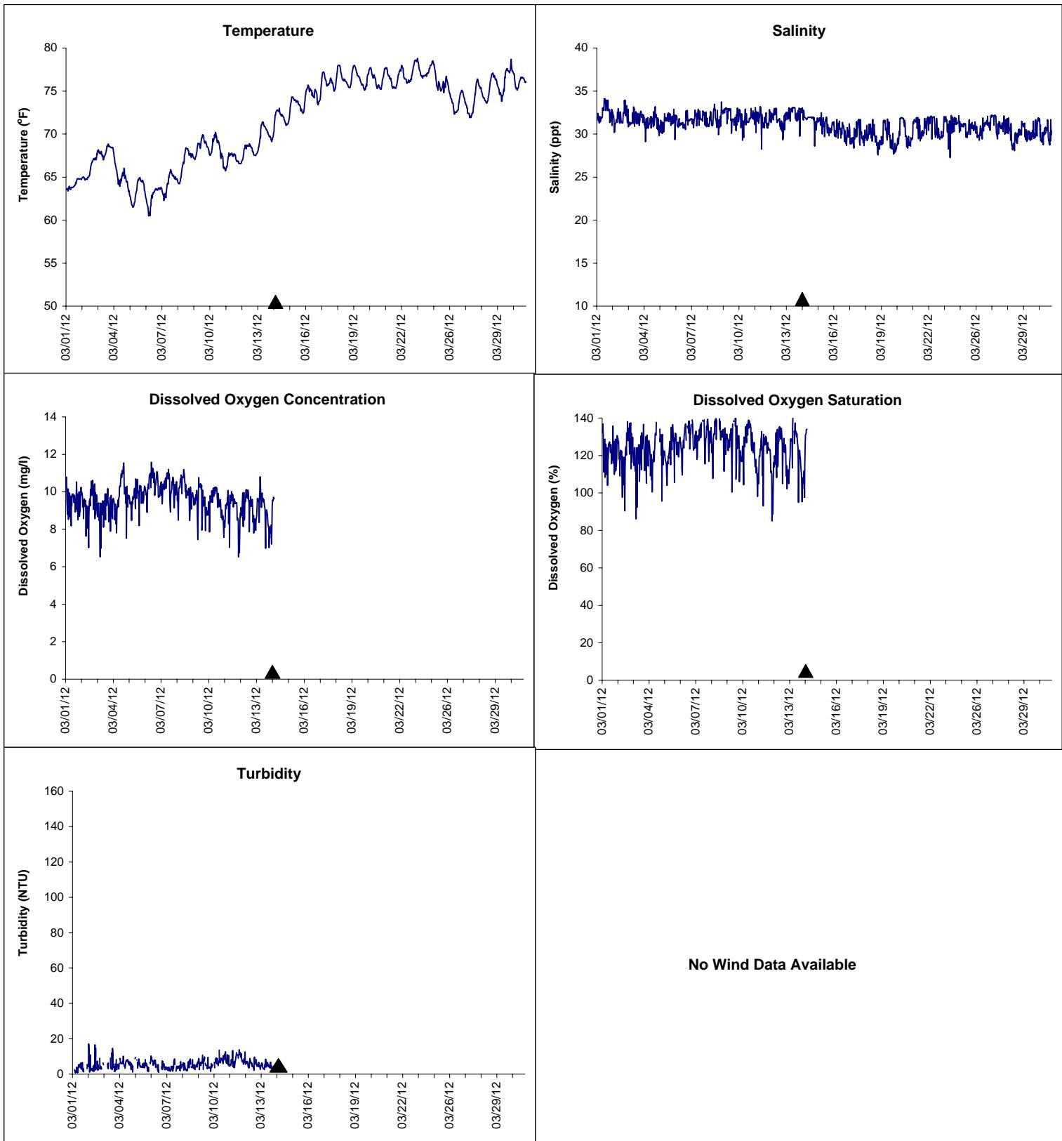
▲ Monitoring Equipment Exchanged (sonde deployment)
