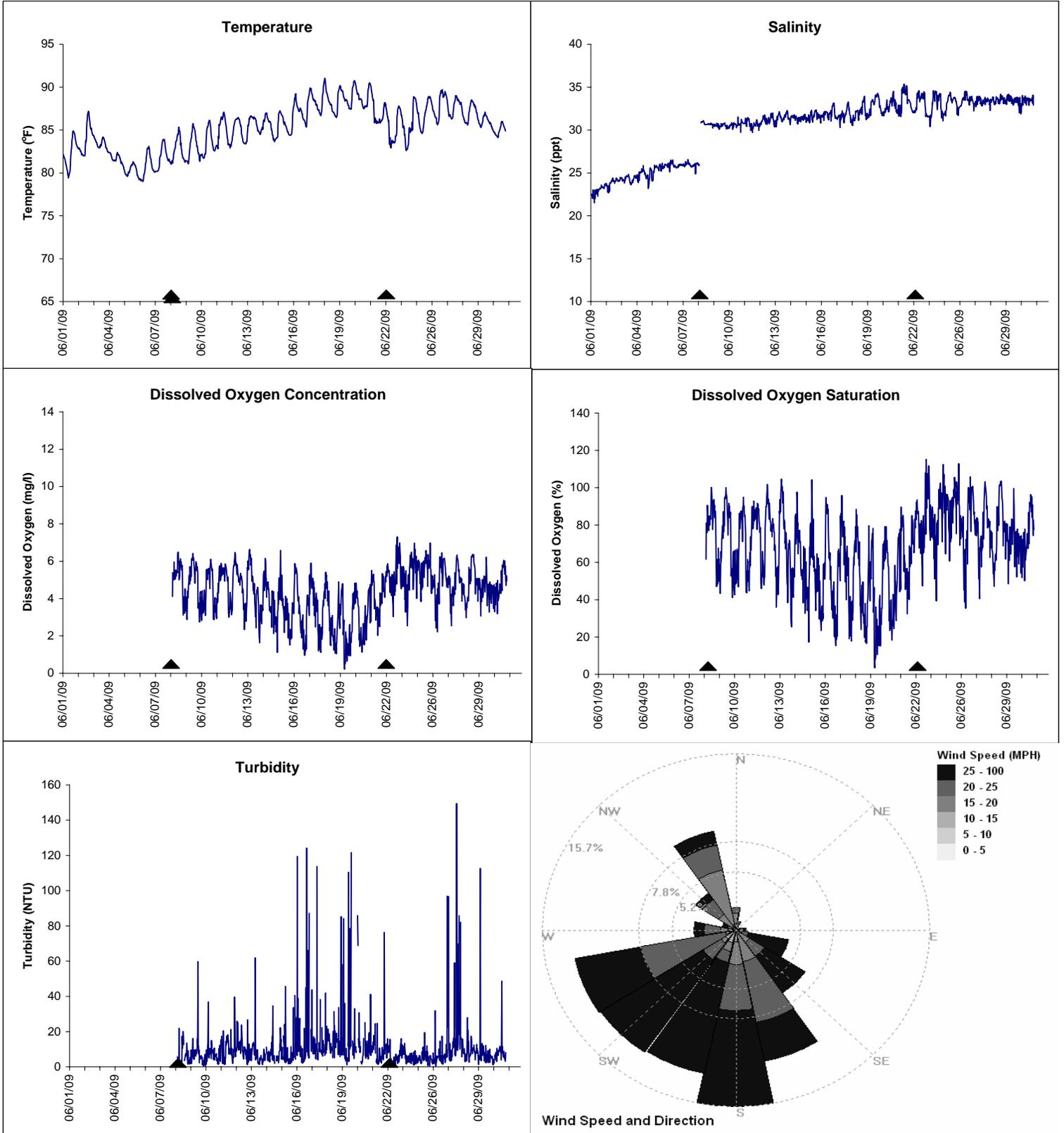
▲ Monitoring Equipment Exchanged (sonde deployment)
