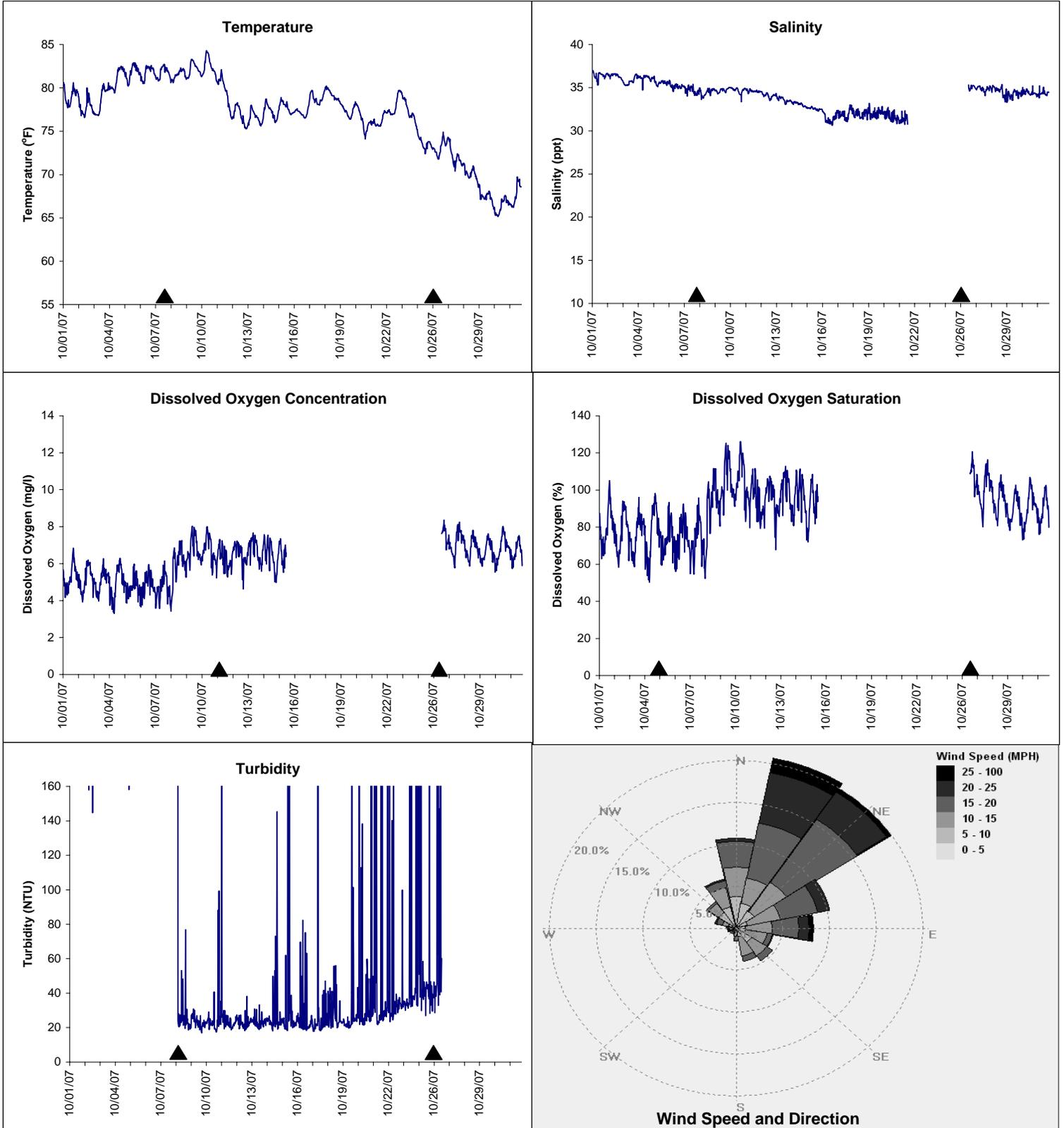
▲ Monitoring Equipment Exchanged (sonde deployment)
