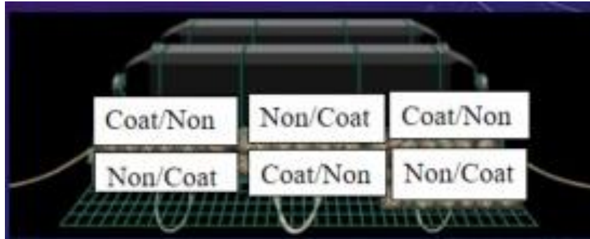
Figure 8. Design of oyster growing bags with and without antifouling fouling coatings inside growing cages.
