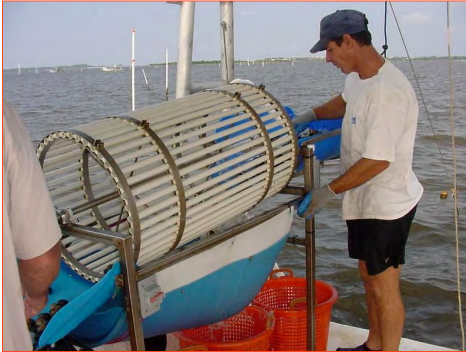
Tumbler on boat – washing clams at lease area
