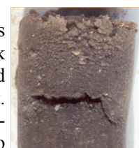
Sediment core sample from a lease. The black area is the anoxic sediment where hydrogen sulfide can be found.
