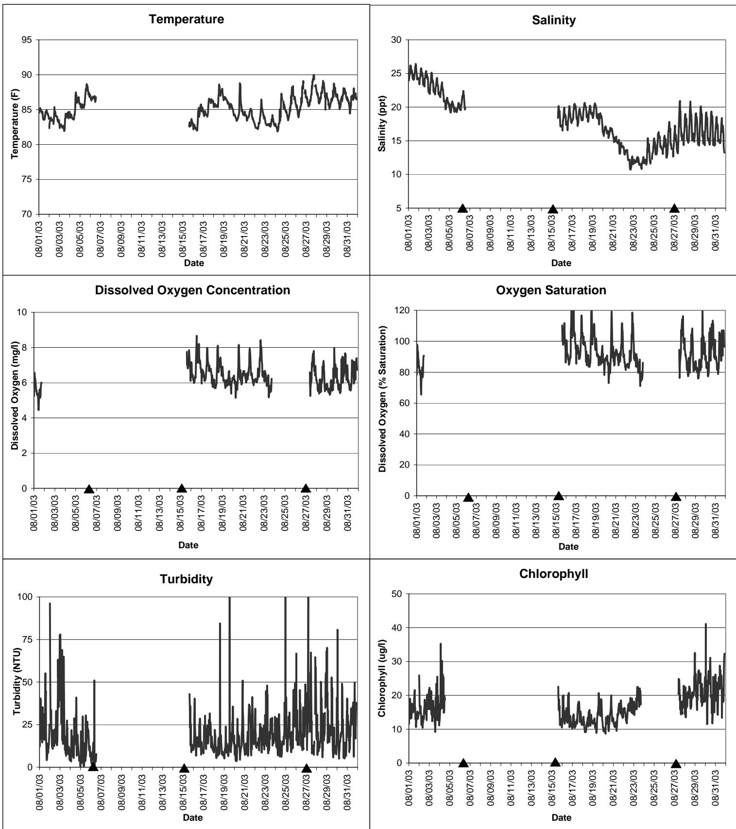
▲ Monitoring equipment exchanged (sonde deployment).
