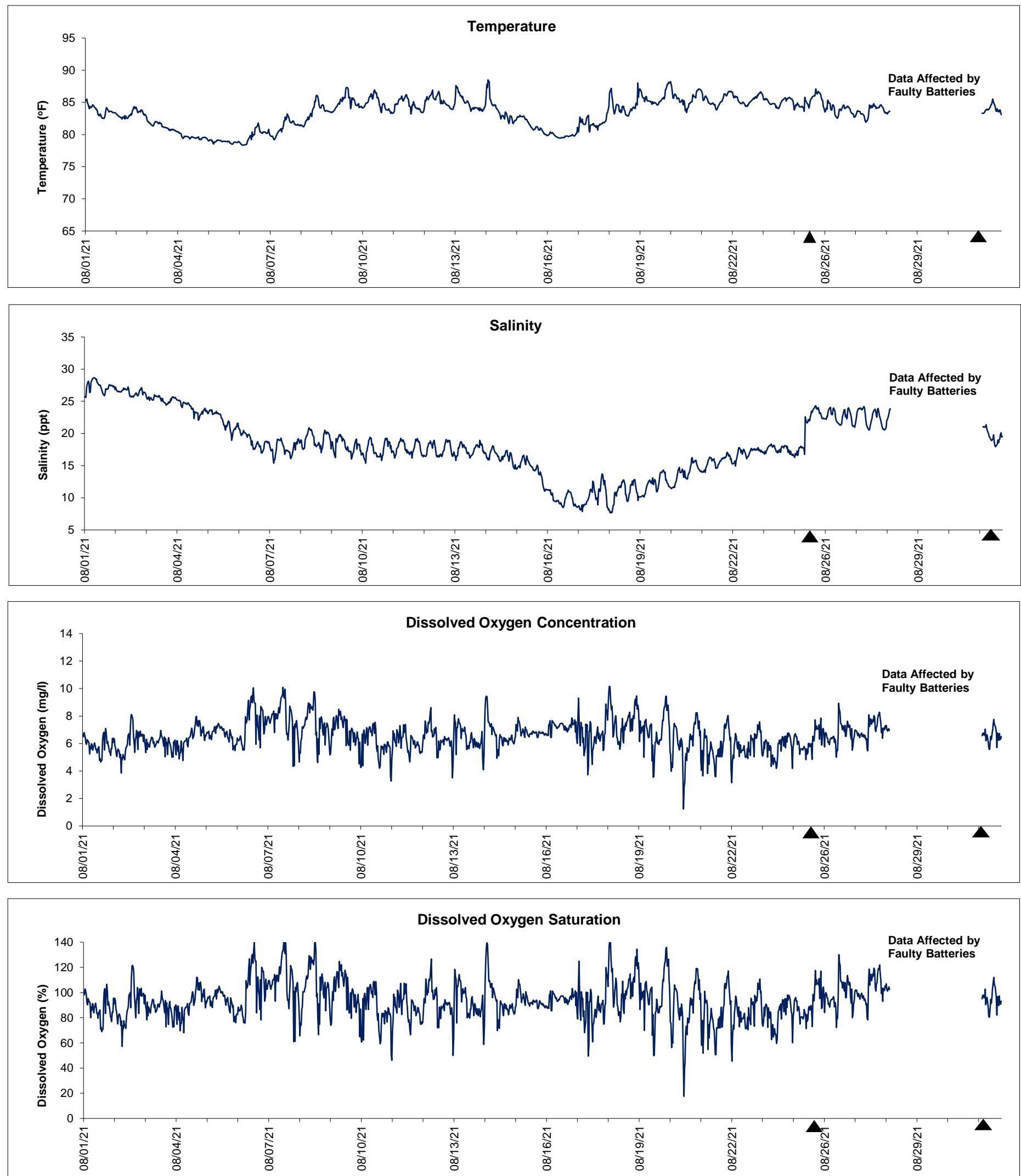
▲ Monitoring Equipment Exchanged (sonde deployment)
