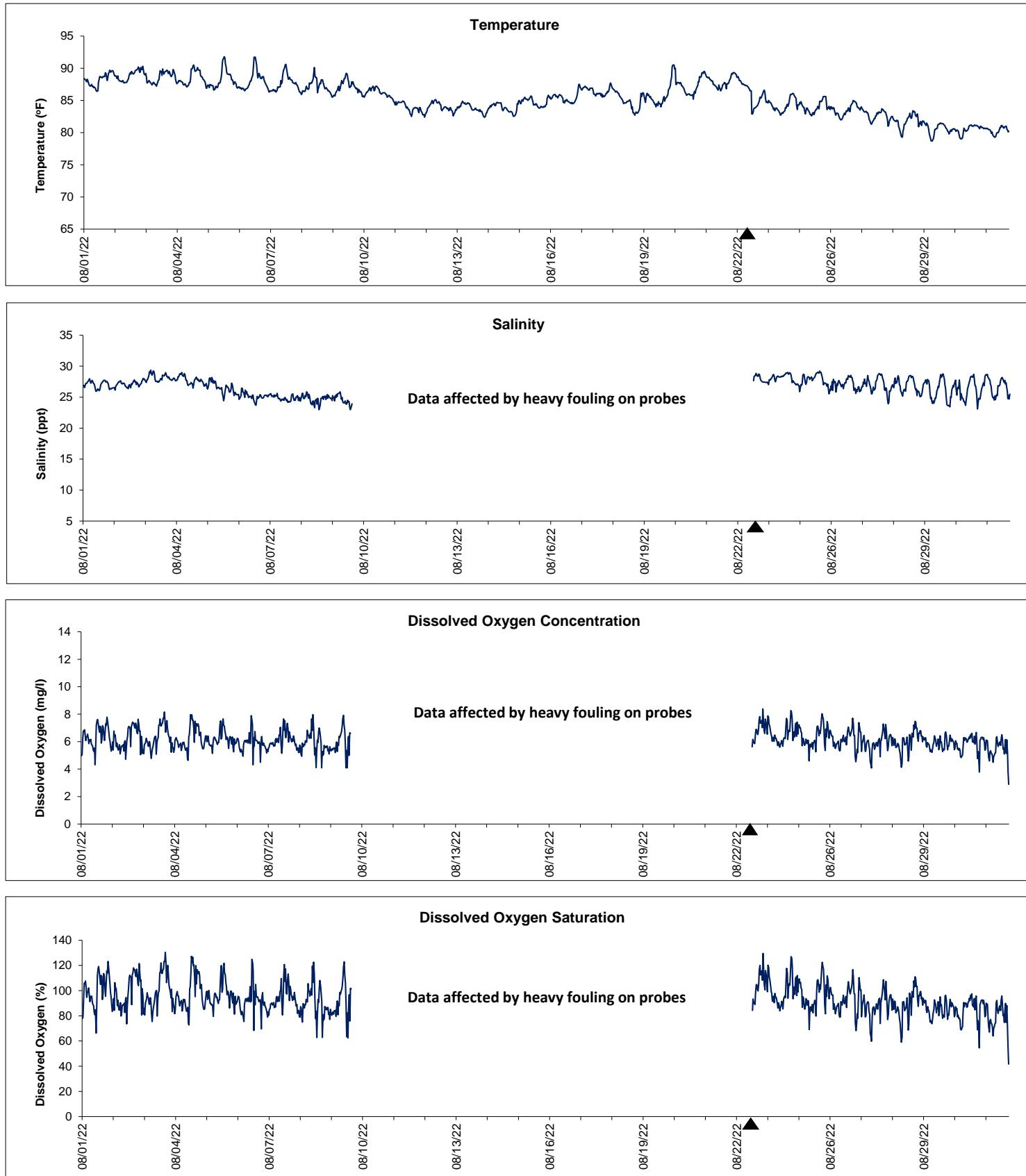
▲ Monitoring Equipment Exchanged (sonde deployment)
