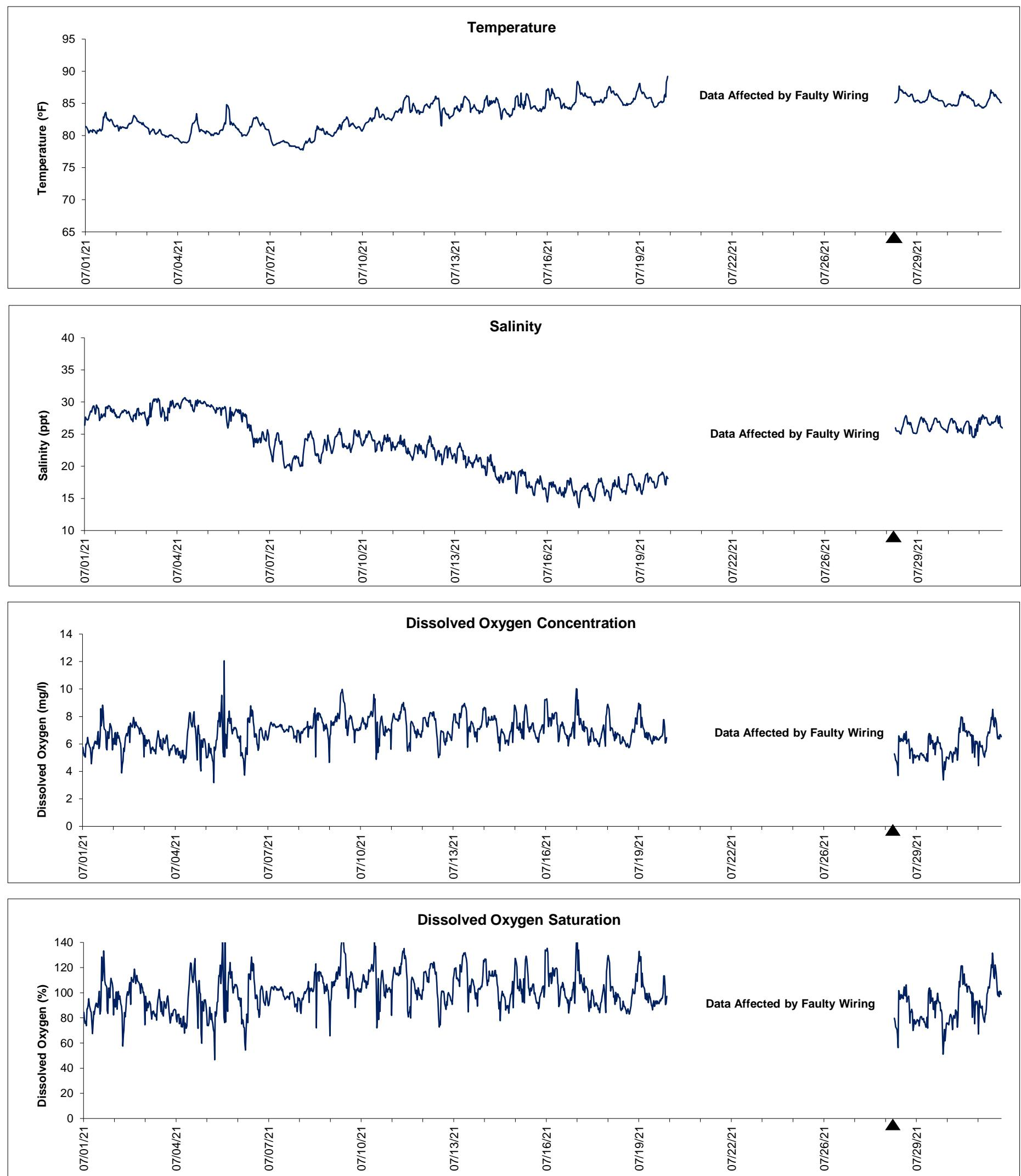
▲ Monitoring Equipment Exchanged (sonde deployment)
