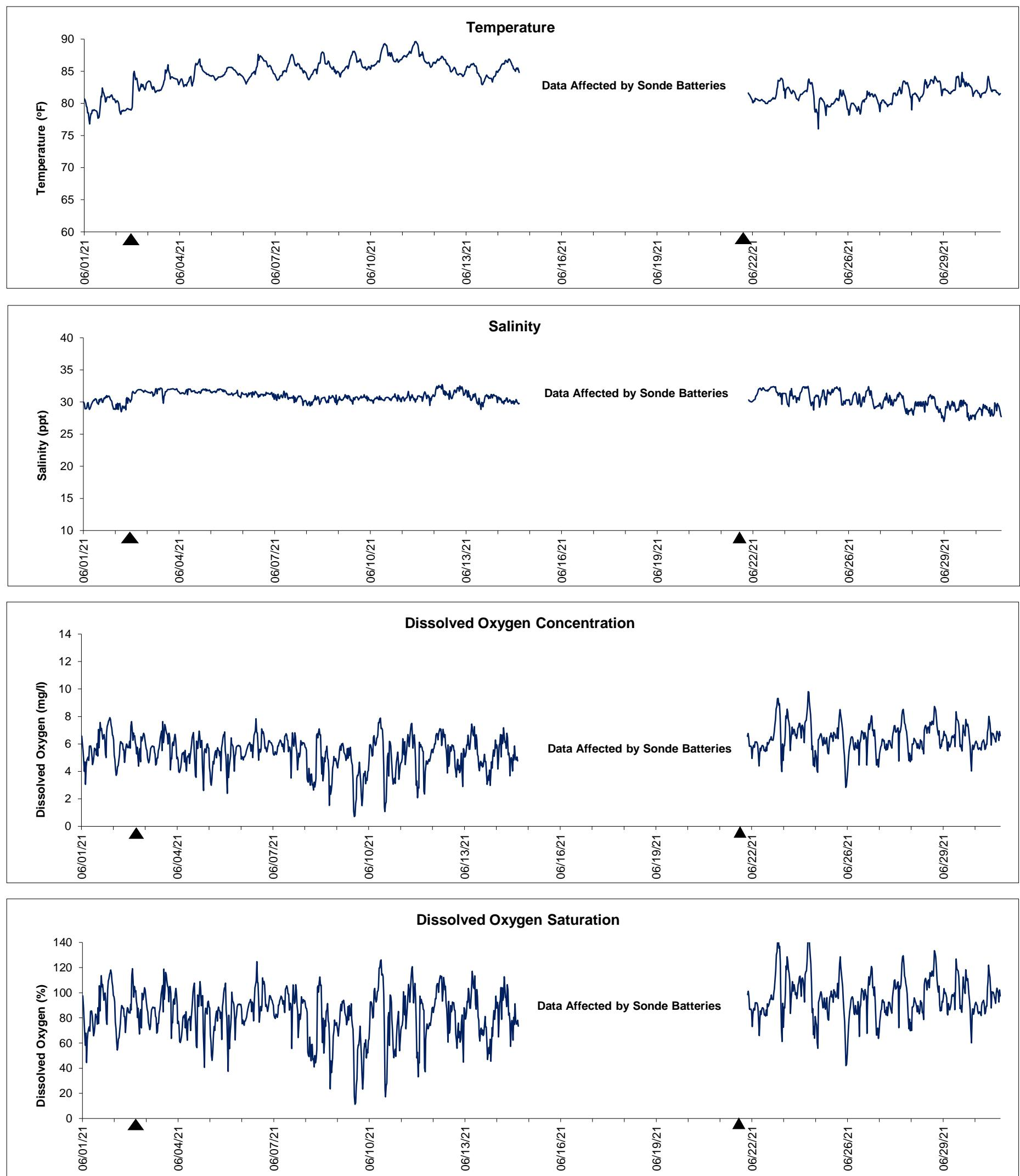
▲ Monitoring Equipment Exchanged (sonde deployment)
