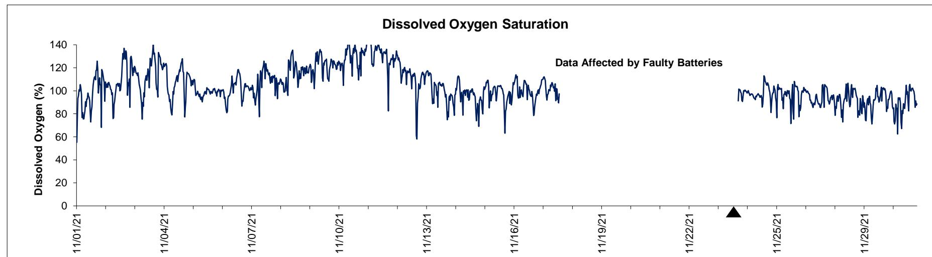
▲ Monitoring Equipment Exchanged (sonde deployment)
