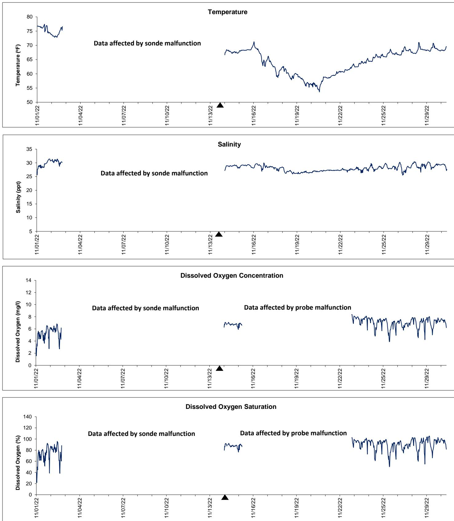
▲ Monitoring Equipment Exchanged (sonde deployment)
