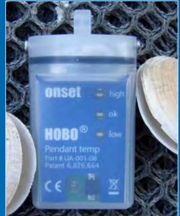
HOBO® Pendant Temperature Data Logger (2.3 x 1.3 x 0.9 inches)
