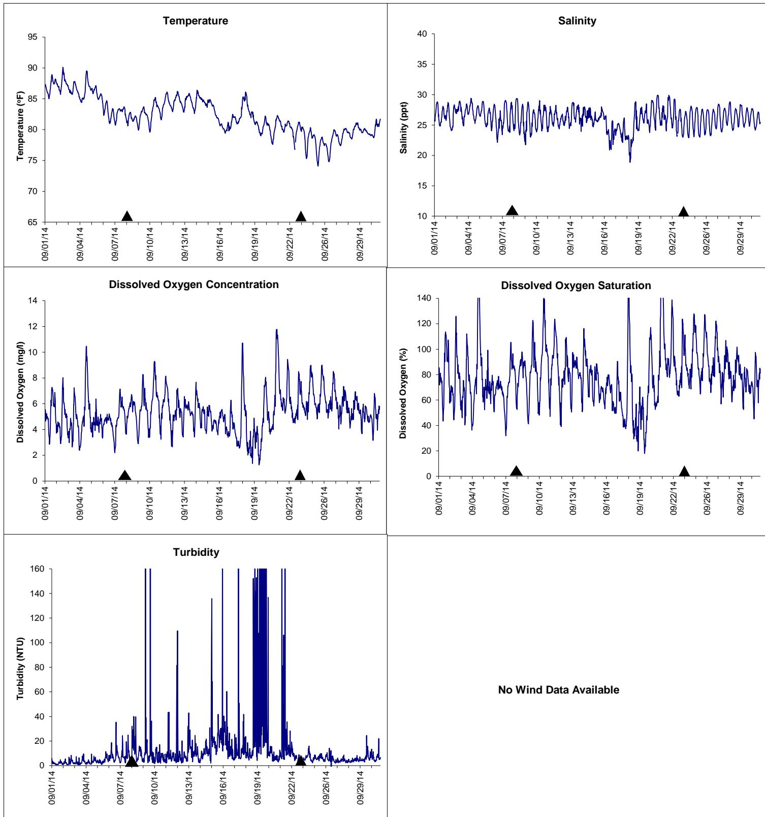
▲ Monitoring Equipment Exchanged (sonde deployment)
