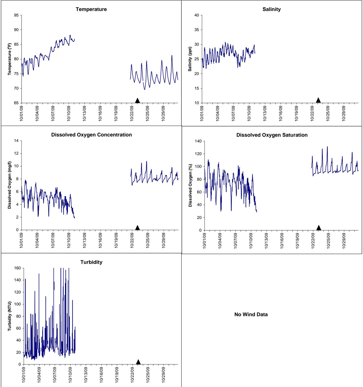
▲ Monitoring Equipment Exchanged (sonde deployment)
