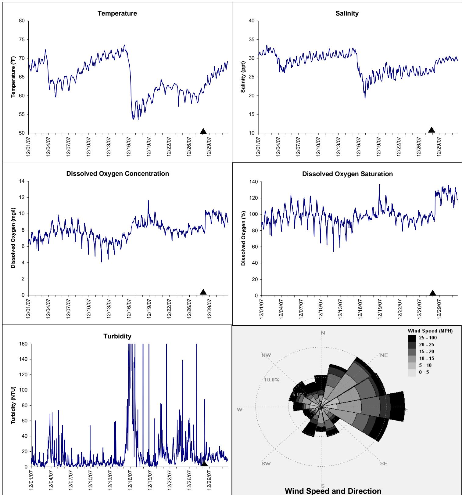
▲ Monitoring Equipment Exchanged (sonde deployment)
