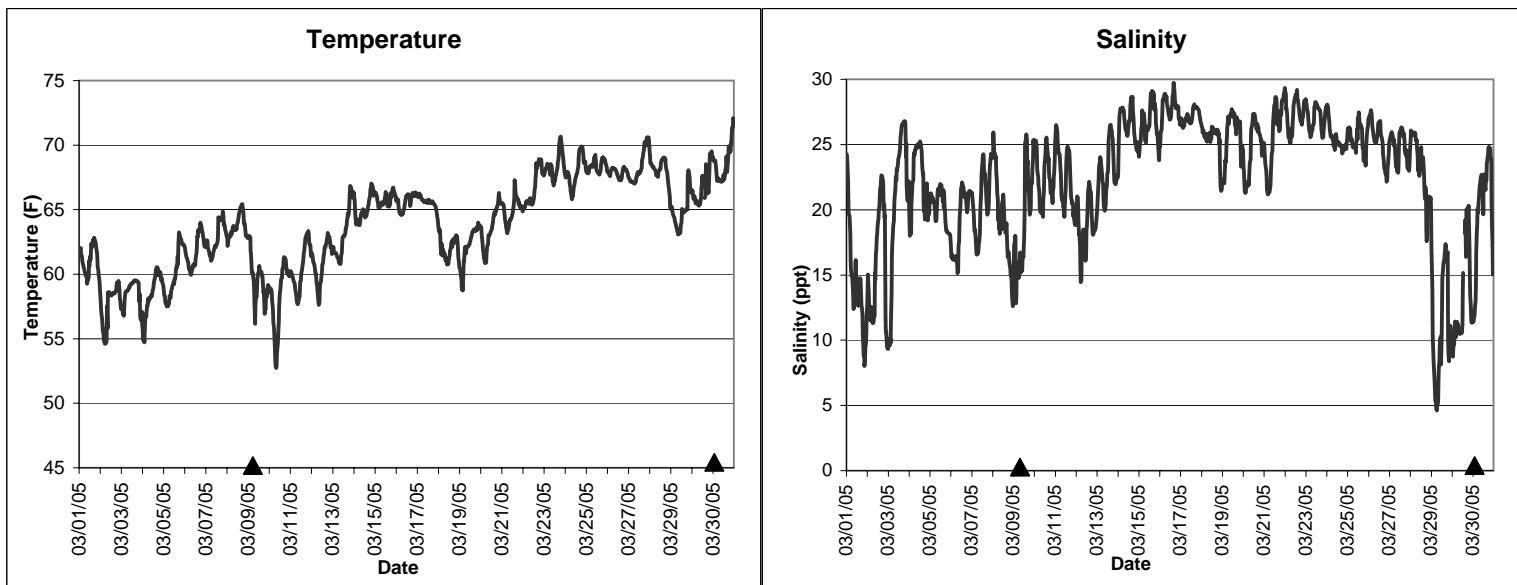
▲ Monitoring equipment exchanged (sonde deployment)
