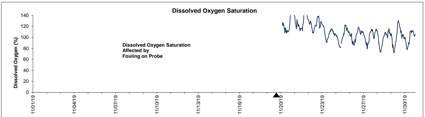
▲ Monitoring Equipment Exchanged (sonde deployment)
