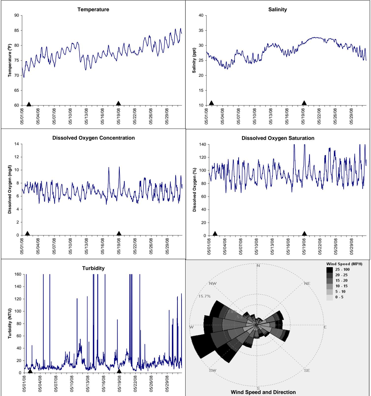
▲ Monitoring Equipment Exchanged (sonde deployment)
