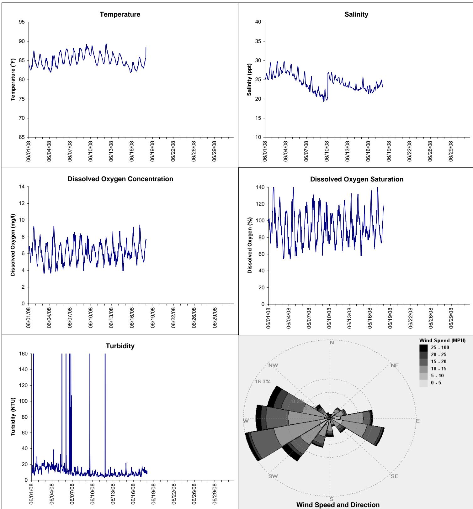
▲ Monitoring Equipment Exchanged (sonde deployment)
