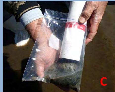
**5. Allow time for the contents of the bag to settle before pouring off any clear water. Seal the bag securely. Place the three soil sample bags from each 2.0-2.5 acre area into a gallon bag. Make sure the bags have been properly labeled with name, lease number, sample number, and date sampled.**
