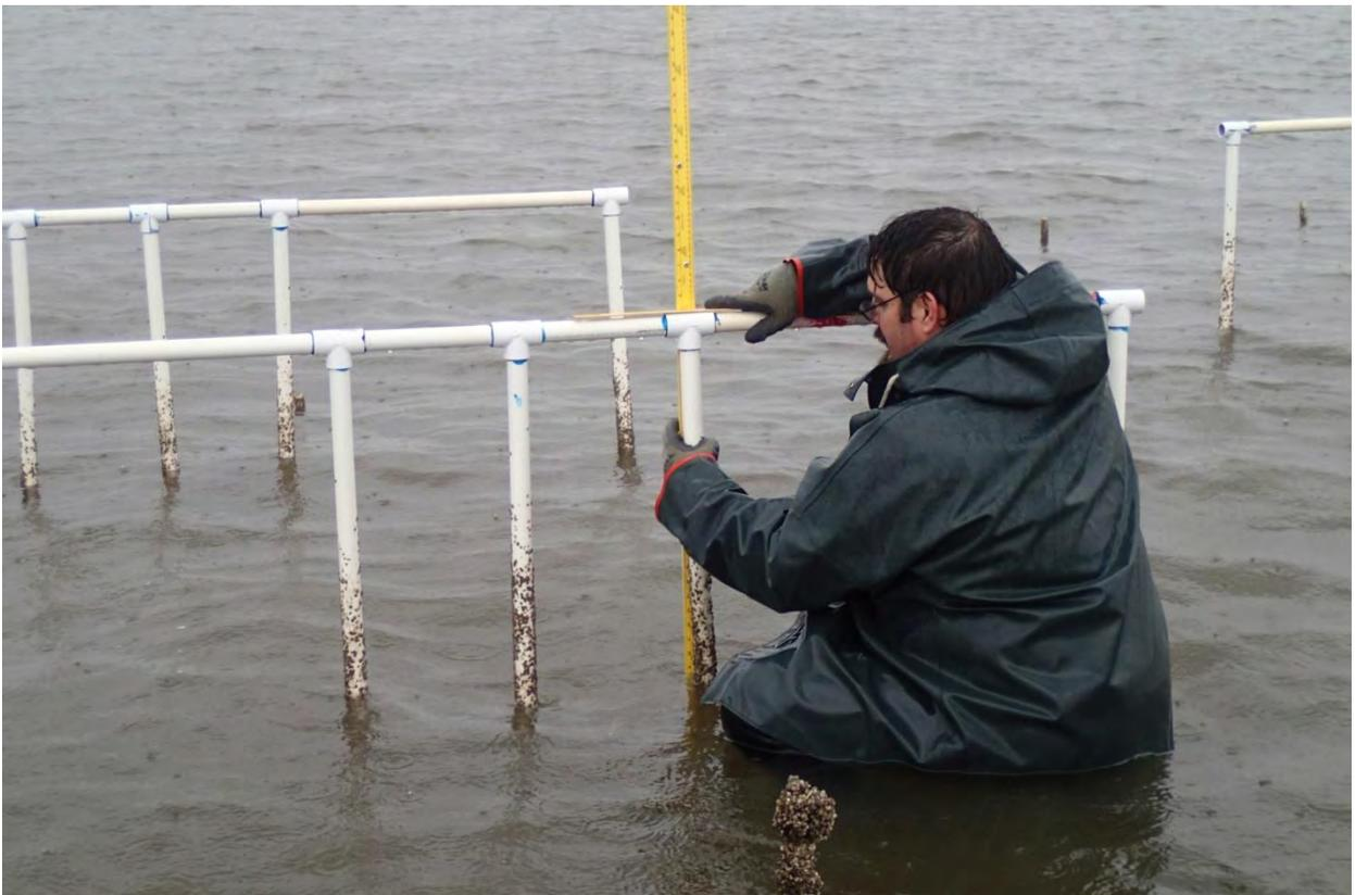
**Figure 8.** PVC pipe arrays were used to measure soil elevations for determining the extent of the harvest tracks from the bottom plant and bags and to monitor recovery of the soils over time.
