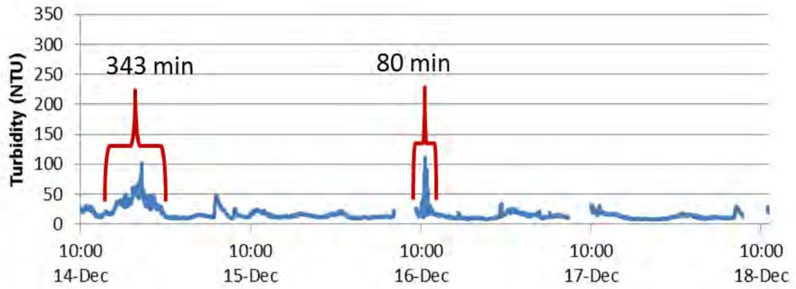
**Figure 17.** Example of duration of natural background turbidity (353 min) in relation to combined bag and bottom plant harvests (80 min).
