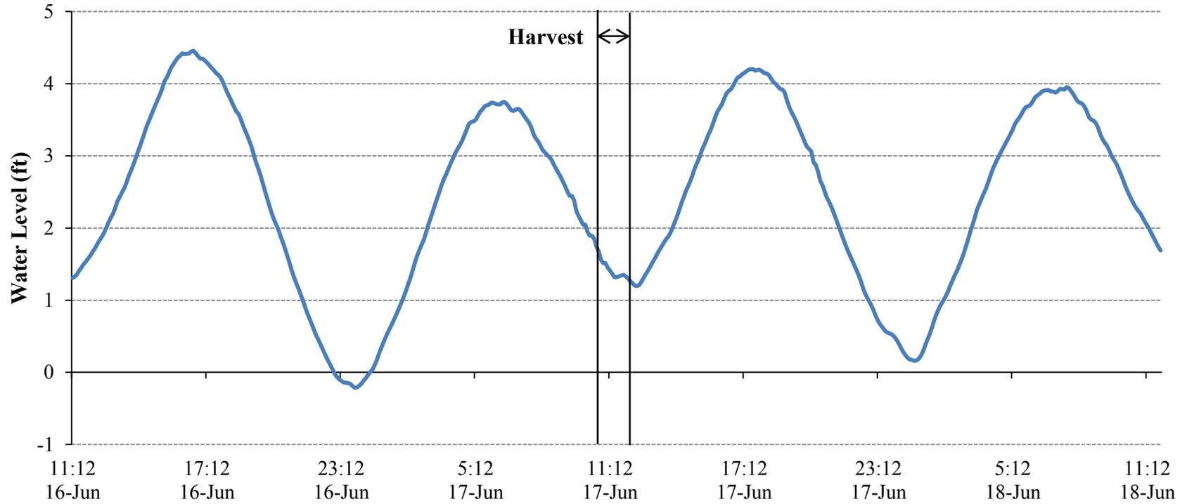
**Figure 18.** Tidal fluctuations measured at the city dock in Cedar Key, Florida (NOAA station 8727520) during harvest (17 June 2014, 10:52-11:46am) and 24 hours pre-and post-harvest.
