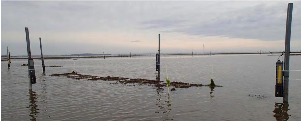
**Figure 3.** Water quality monitoring sondes positioned around a bottom net (above) and bottom bags (below) prior to harvest. Note sondes were exposed during a minus tide on this harvest date (field replicate #3). Harvesting activities did not begin until 30 minutes after the incoming tide inundated the sondes.
