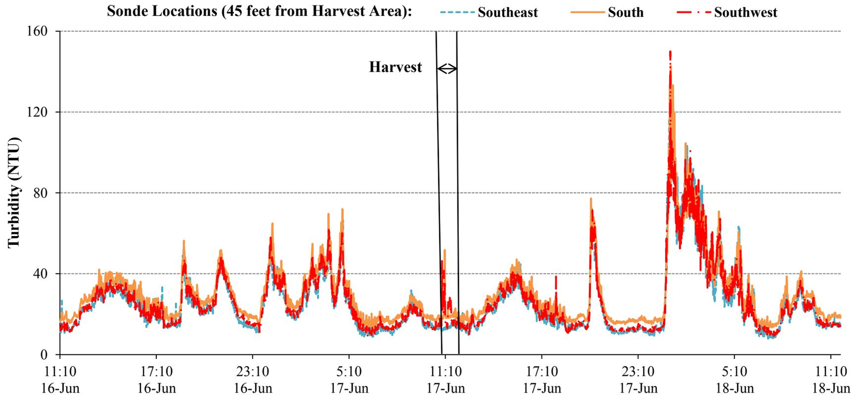
**Figure 21.** Turbidity (NTU) values at sondes located 45 feet from the commercial test area during harvest (17 June 2014, 10:52-11:46am) and 24-hours pre- and post-harvest.
