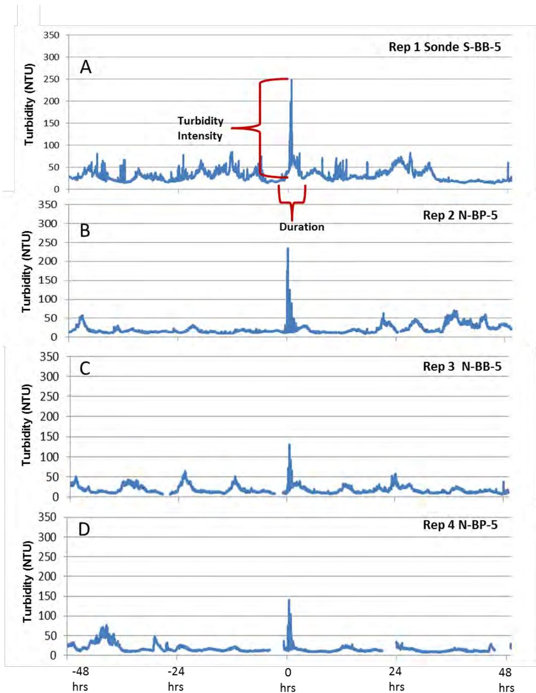
**Figure 11.** Corrected turbidity measurements (NTU) for 48 hours pre and post of each of four combined bag and bottom plant harvest replicates. Center peak is the intensity of the harvest activity (time 0). Note duration of harvest event (red close bracket) in relation to other natural events. (A) indicates experimental replicate 1, (B) replicate 2, (C) replicate 3, and (D) replicate 4.
