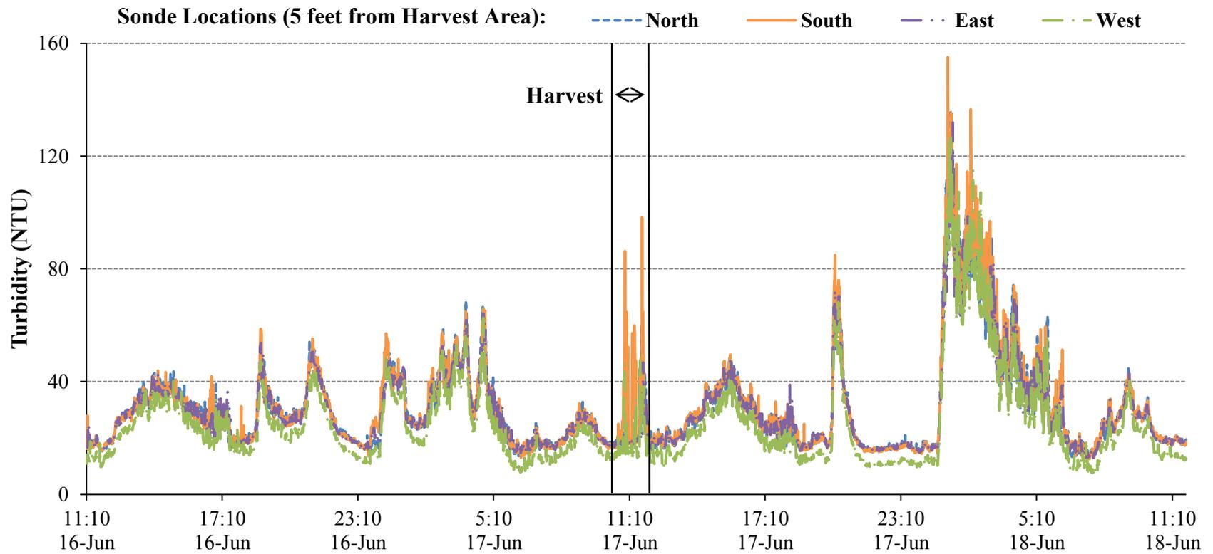
**Figure 19.** Turbidity (NTU) values at sondes located five feet from the commercial test area during harvest (17 June 2014, 10:52-11:46am) and 24-hours pre- and post-harvest.
