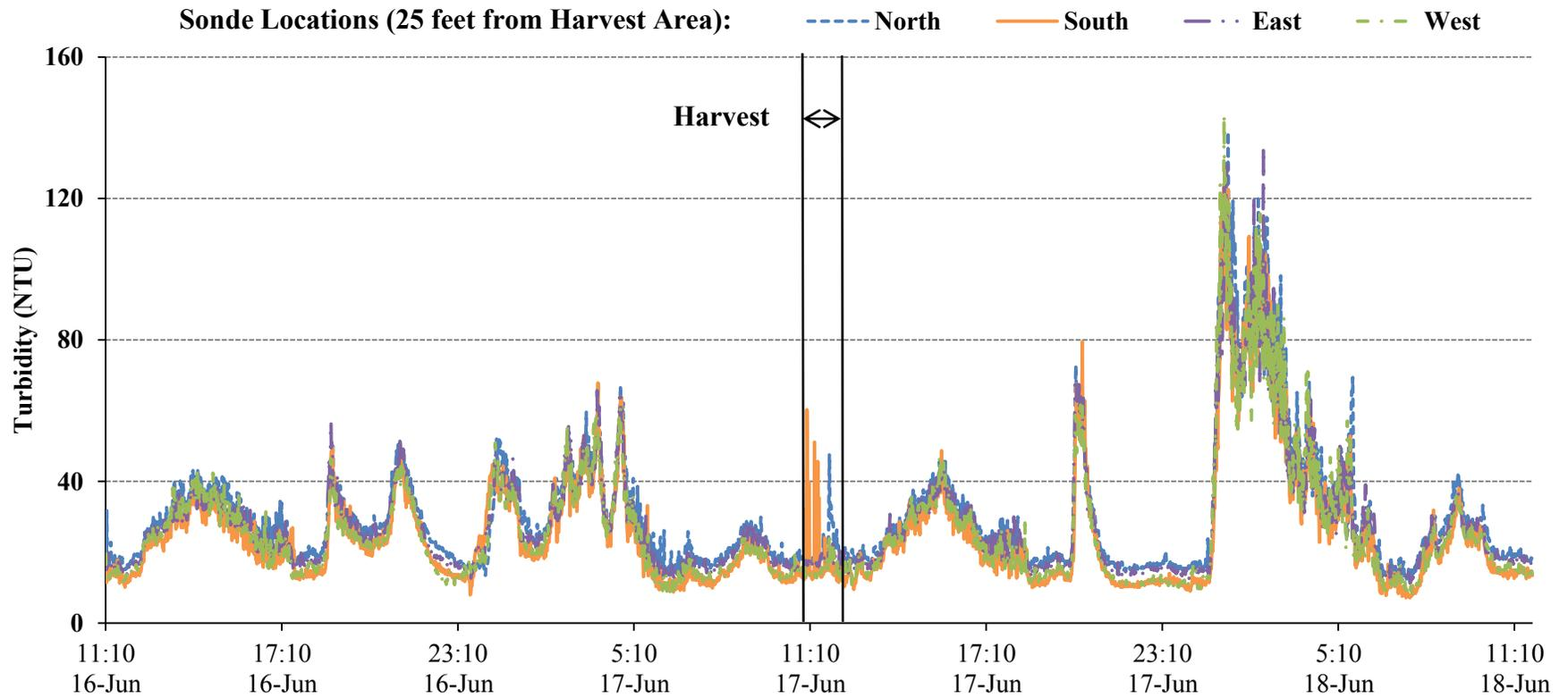
**Figure 20.** Turbidity (NTU) values at sondes located 25 feet from the commercial test area during harvest (17 June 2014, 10:52-11:46am) and 24-hours pre- and post-harvest.
