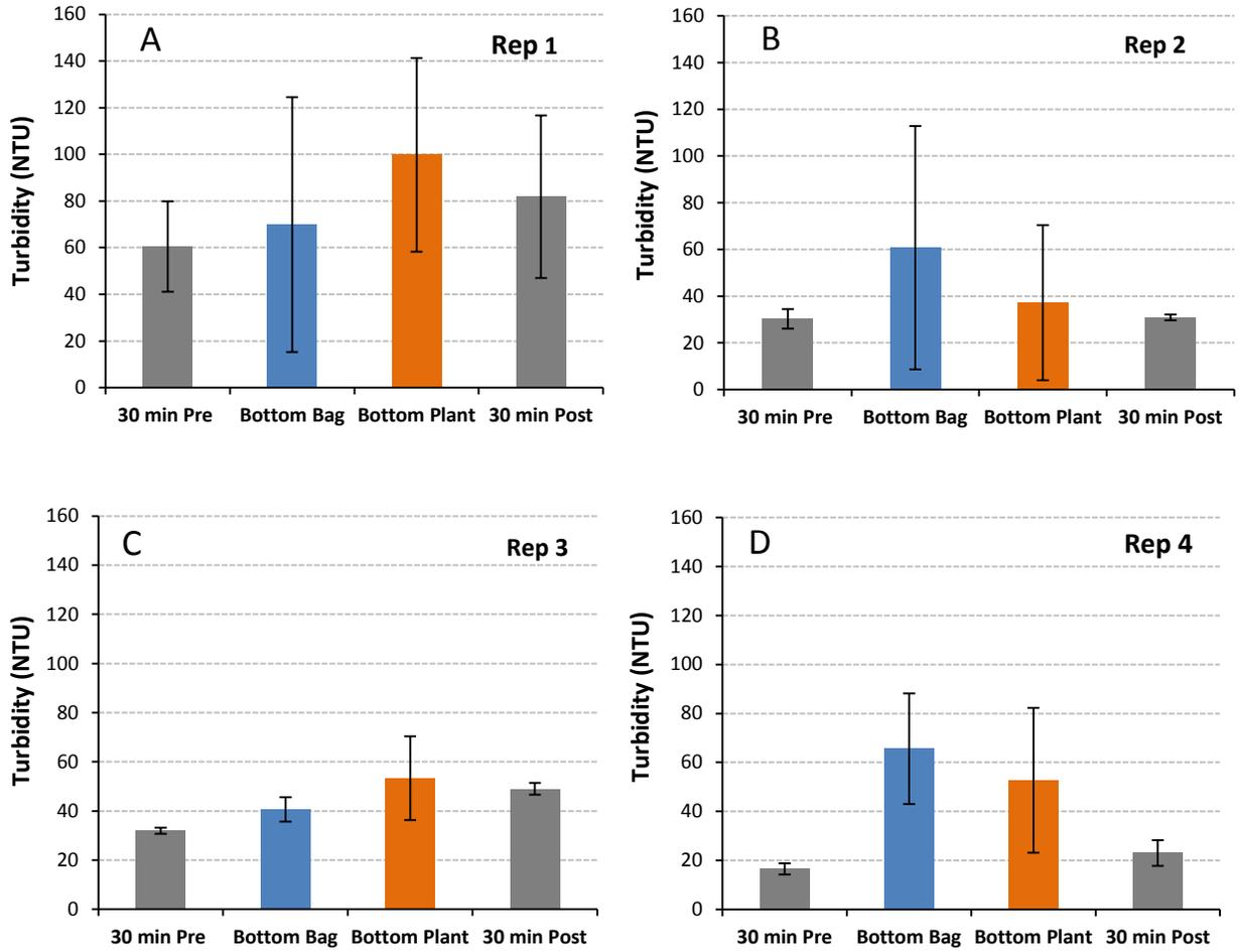
**Figure 12.** Comparison of highest mean turbidity observations for 30 minutes pre-harvest, bottom bag harvest, bottom plant harvest, and 30 minutes post-harvest. (A) indicates experimental replicate 1, (B) replicate 2, (C) replicate 3, and (D) replicate 4.
