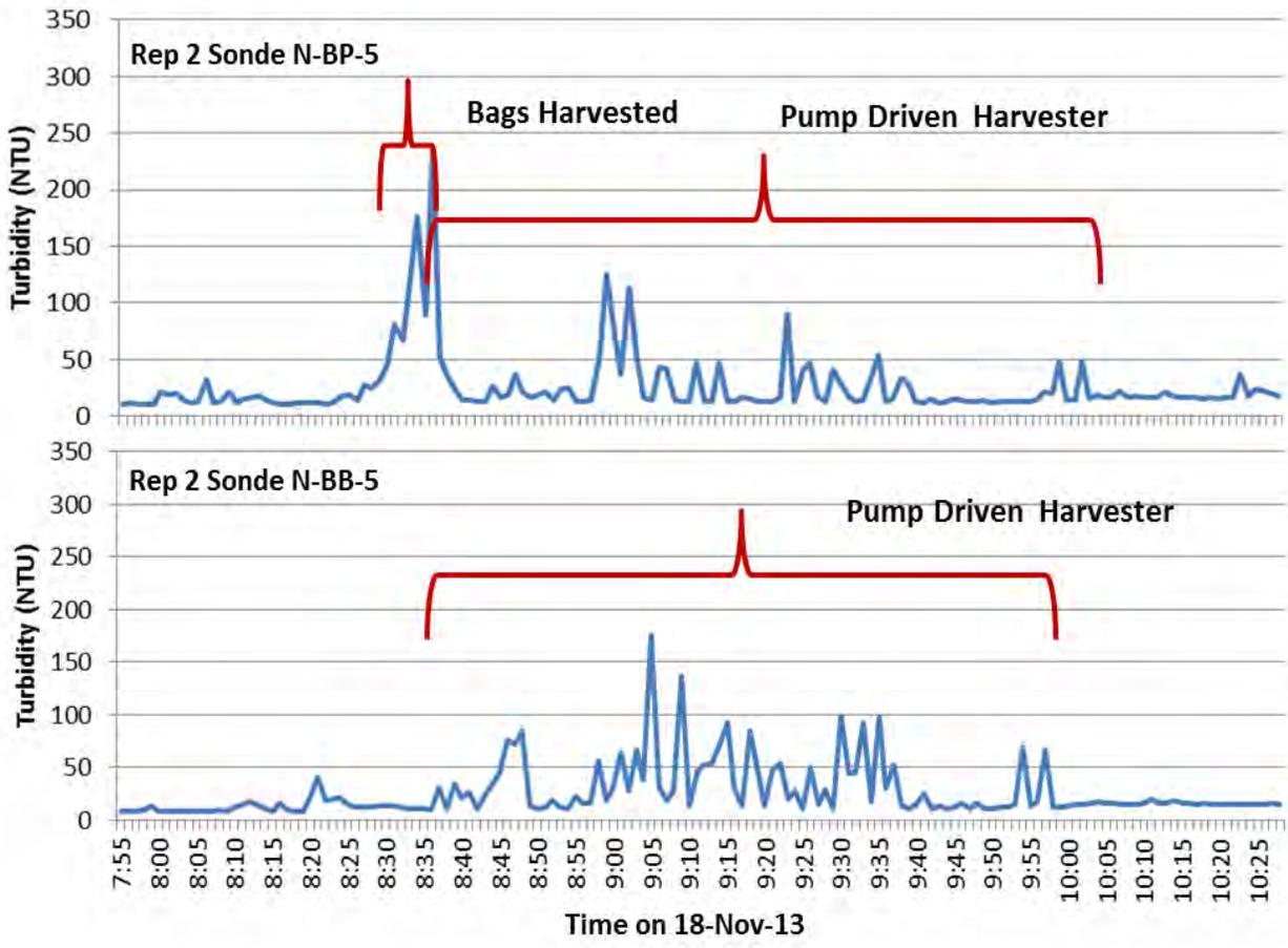
**Figure 14.** Comparison of bag harvest (top graph) and pump-driven harvester (bottom graph) from replicate 2. Return interval for turbidity associated with harvesting the bags was not determined; however, turbidity associated with the use of the pump-driven harvester returned to background in 9 minutes in this replicate. Brackets denote the time frame of harvest activity.
