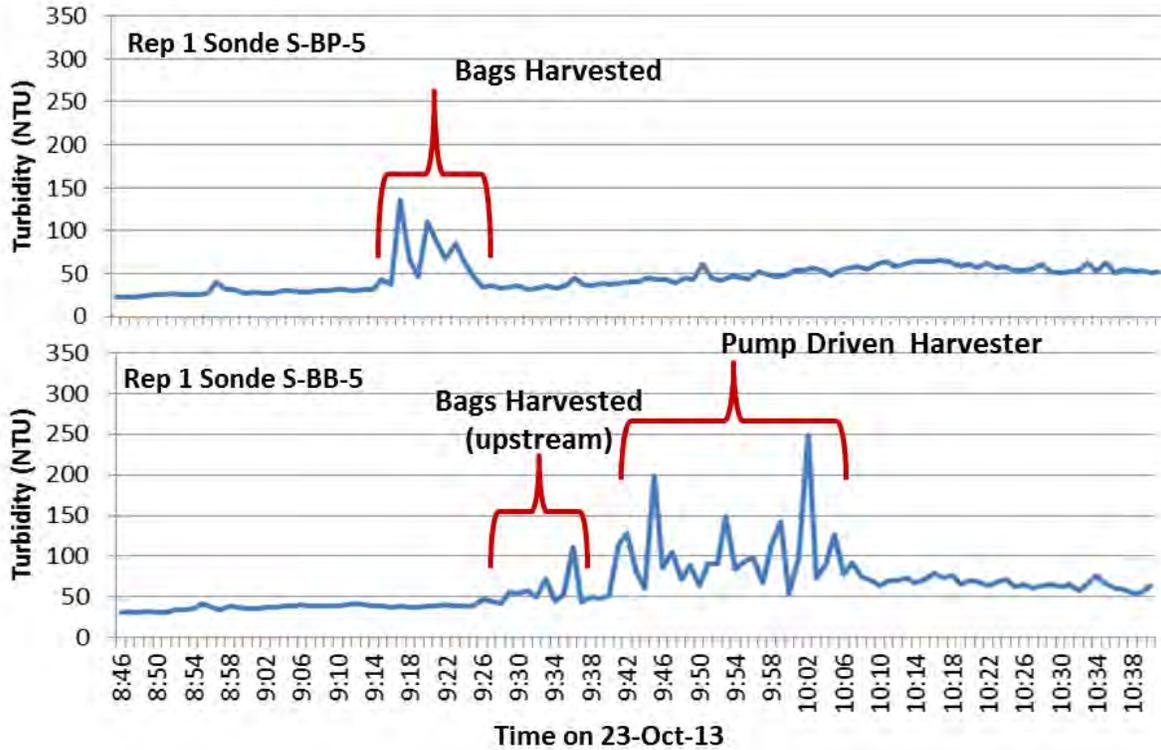
**Figure 13.** Comparison of bag harvest (top graph) and pump-driven harvester (bottom graph) from replicate 1. Turbidity associated with harvesting the bags was determined to return to background level in 2 minutes, while turbidity associated with the use of the pump-driven harvester returned to background in 5 minutes in this replicate. Brackets denote the time frame of harvest activity. Note that due to environmental conditions, the pump harvest was not captured by the S-BP-5 sonde.
