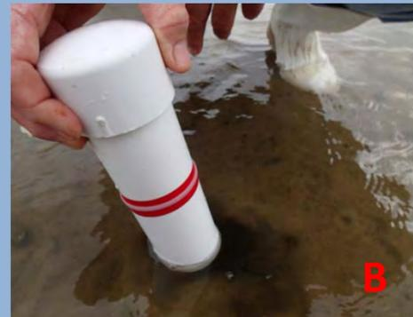
**3. Push the tube over to one side until the bottom breaks free. Immediately cap the bottom of the pipe before bringing the sample to the surface.**
