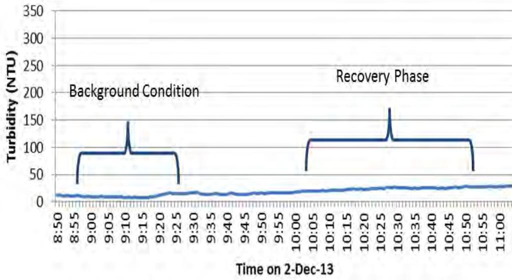
**Figure 5.** Example of baseline correction using turbidity measurements from Sonde W-BP-5 during field replicate 3. Notice the baseline turbidity increases over the course of the tide in the recovery phase. This changing baseline was subtracted from the post-harvest turbidity values to remove the increasing trend in observations and thus accurately determine the return interval.
