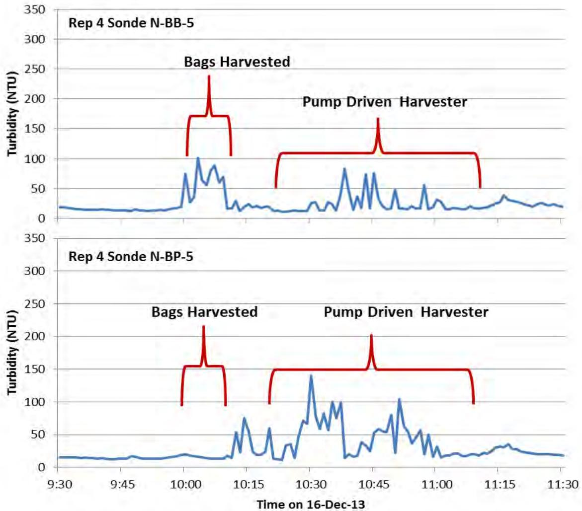
**Figure 16.** Comparison of bag harvest (top graph) and pump-driven harvester (bottom graph) from replicate 4. Turbidity associated with harvesting the bags was determined to return to background level in 5 minutes while turbidity associated with the use of the pump-driven harvester returned to background in 4 minutes in this replicate. Brackets denote the time frame of harvest activity.
