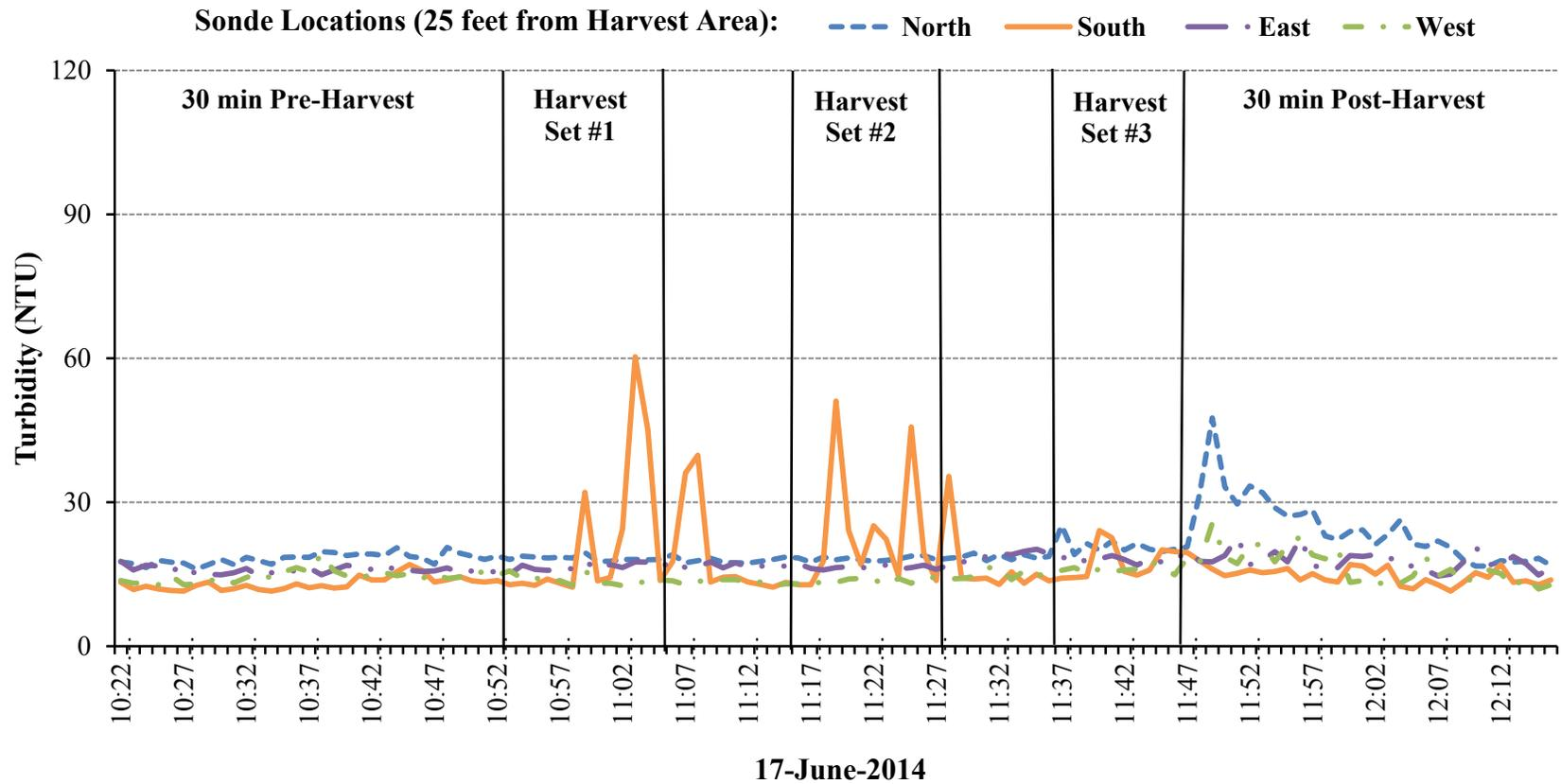
**Figure 24.** Turbidity (NTU) values at sondes located 25 feet from the commercial test area during harvest (17 June 2014, 10:52-11:46am) and 30 minutes pre- and post-harvest. Each harvest set consisted of eight passes of the pump-driven harvester over the test area.
