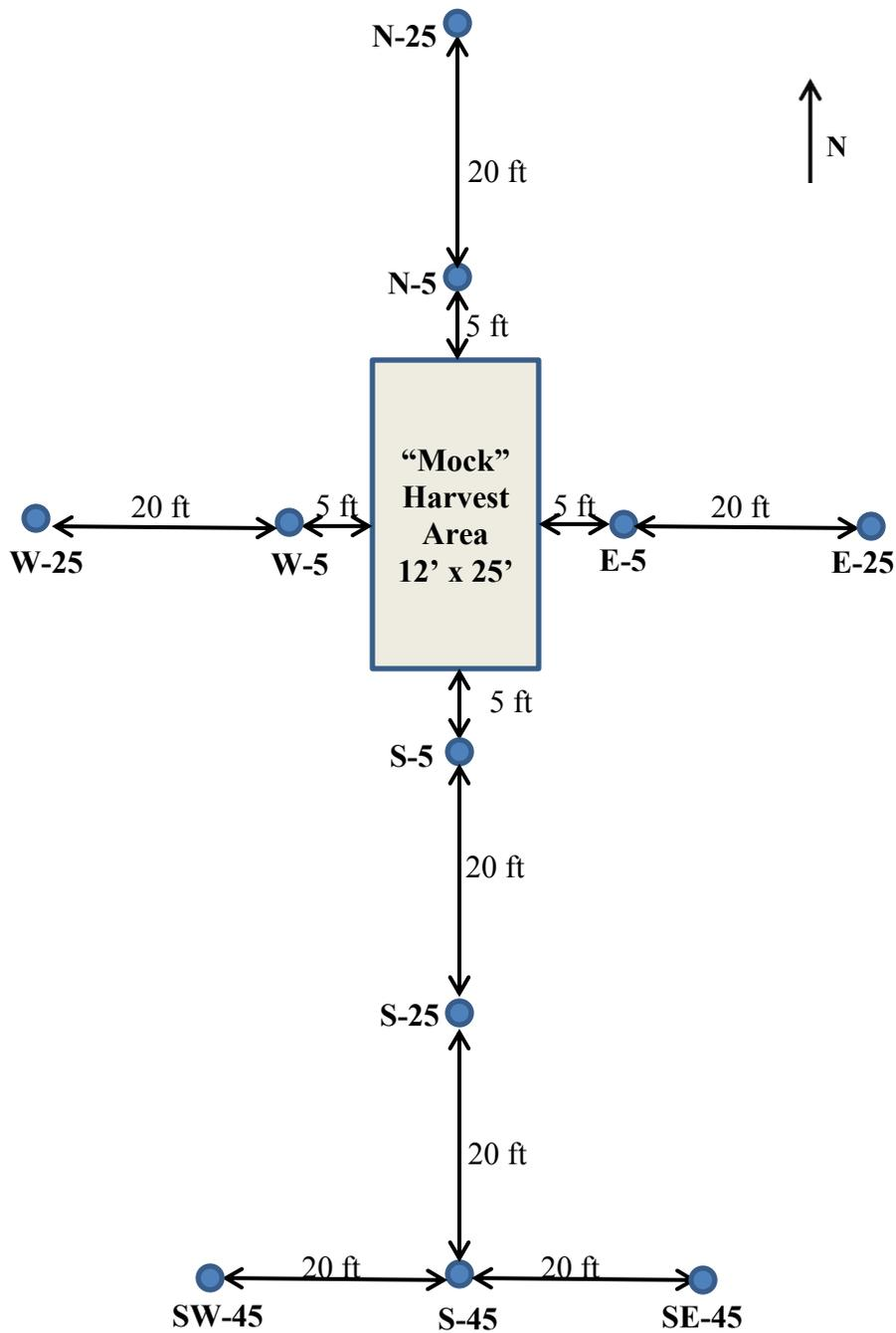
**Figure 6.** Sondes were located at 5 and 25 feet intervals from the commercial-scale harvest area to the north, south, east, and west. Three sondes were also positioned 45 feet south of the harvest area to capture the turbidity plume associated with an outgoing tide. Sonde position is noted as direction and distance from the harvest area (e.g., N-5).
