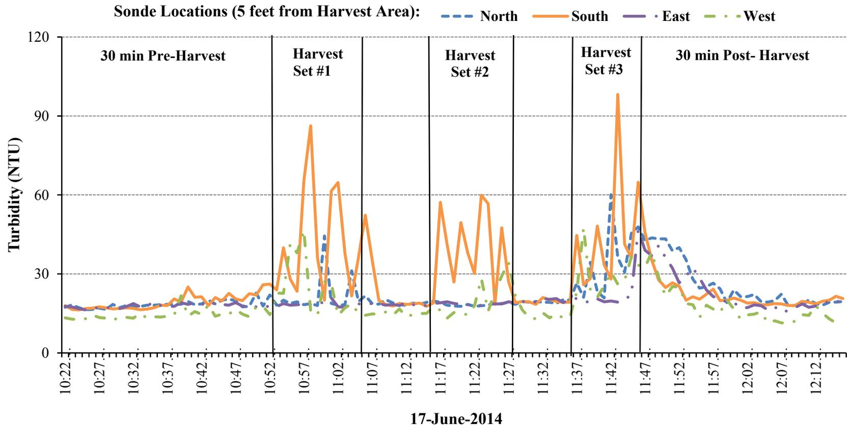
**Figure 23.** Turbidity (NTU) values at sondes located five feet from the commercial test area during harvest (17 June 2014, 10:52-11:46am) and 30 minutes pre- and post-harvest. Each harvest set consisted of eight passes of the pump-driven harvester over the test area.
