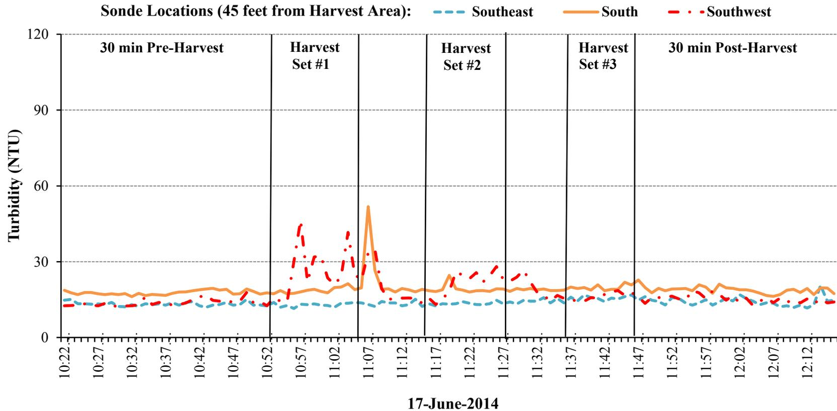
**Figure 25.** Turbidity (NTU) values at sondes located 45 feet from the commercial test area during harvest (17 June 2014, 10:52-11:46am) and 30 minutes pre- and post-harvest. Each harvest set consisted of eight passes of the pump-driven harvester over the test area.
