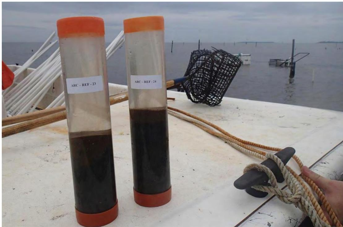
**Figure 7.** Collecting soil cores immediately after harvest to determine soil properties and compare with those established at plant and at adjacent reference (unfarmed) sites.
