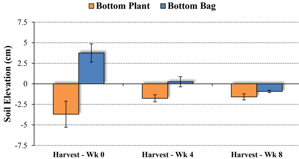
**Figure 28.** Average soil elevations at culture sites (bottom plant and bottom bag) relative to adjacent unfarmed references immediately after harvest (week 0) and 4 and 8 weeks post-harvest. Zero soil elevation represents where average track depth was equal to average reference site elevation. Bars represent standard deviation.
