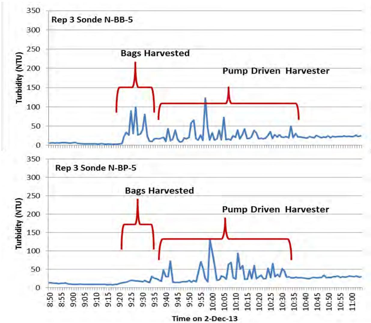
**Figure 15.** Comparison of bag harvest (top graph) and pump-driven harvester (bottom graph) from replicate 3. Return interval for turbidity associated with harvesting the bags was not determined; however, turbidity associated with the use of the pump-driven harvester returned to background in 5 minutes in this replicate. Brackets denote the time frame of harvest activity.
