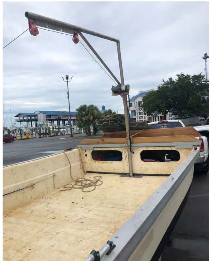
FIGURE 2. A mechanical davit used to raise sunken floating cages from the seafloor after the storm has passed. Photo courtesy of Jason Rider
