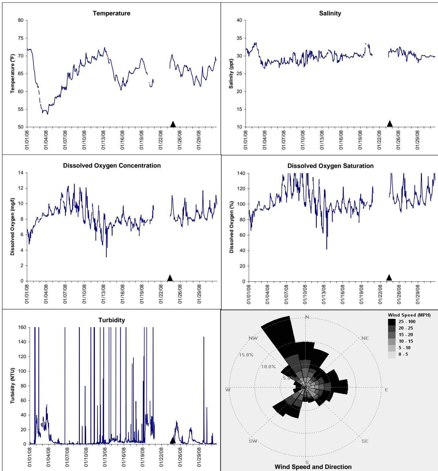
▲ Monitoring Equipment Exchanged (sonde deployment)
