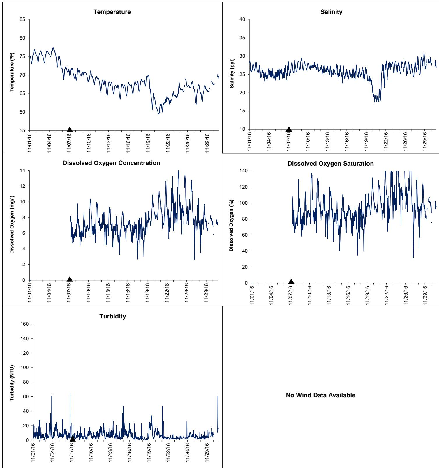
▲ Monitoring Equipment Exchanged (sonde deployment)
