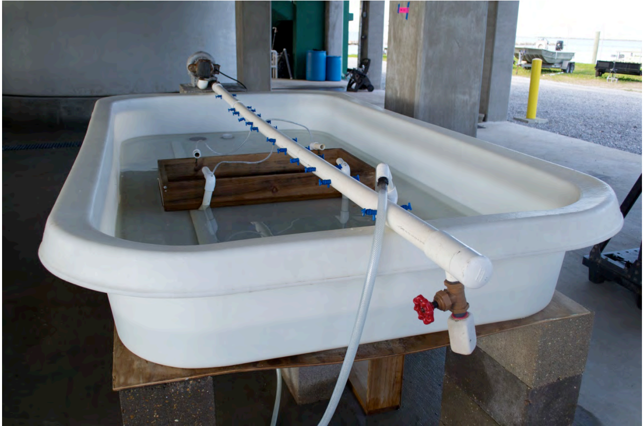
Figure 13. Setting tank. A blower is connected to a manifold that runs along the length of the tank. Flexible rubber tubing connects the manifold to the airlifts attached to setting trays. Water is recirculated from a reservoir by a sump and discharged through a hose positioned at the end opposite the stand-pipe.
