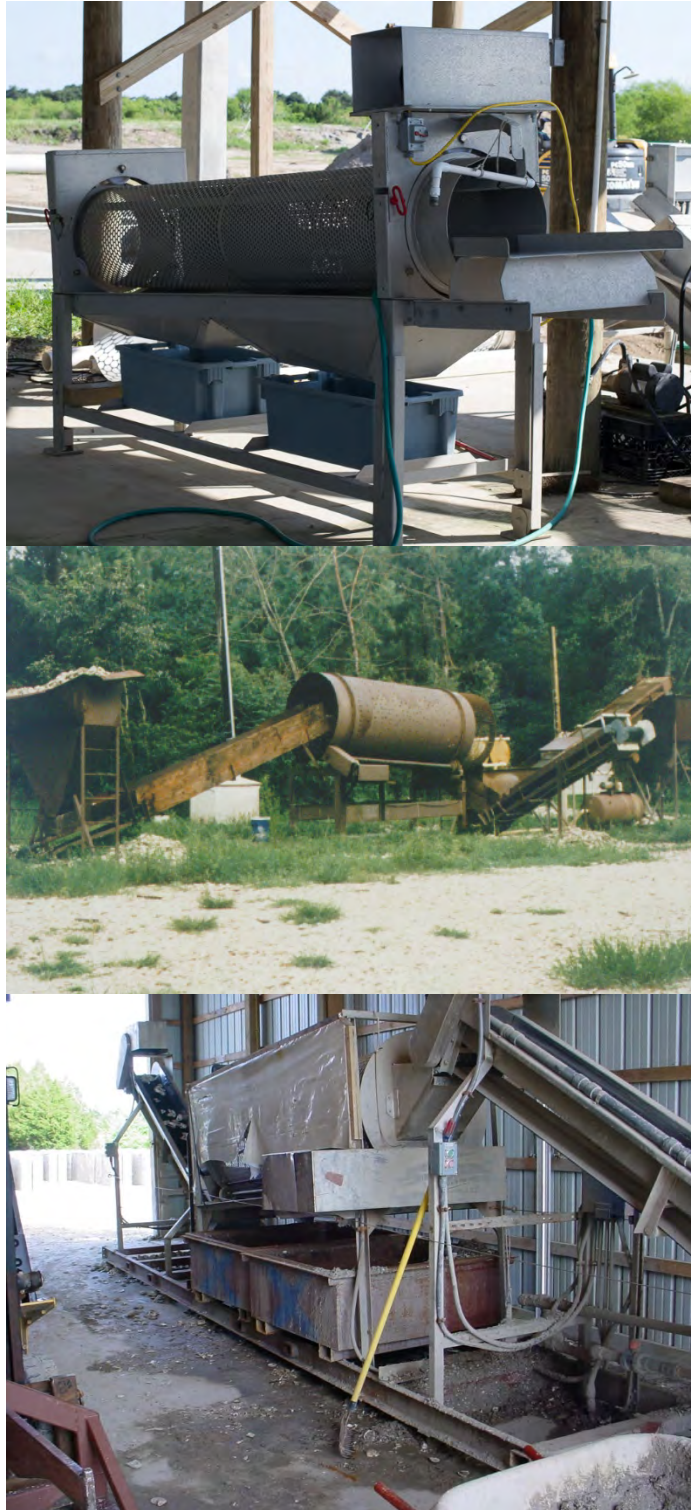
Figure 10. Oyster size graders that can be used to grade and wash seed simultaneously. Seed oysters or cultch materials are loaded into the grader as the drum rotates and water is sprayed into the rotating drum washing shells and allowing oysters/shells to fall through appropriate sized holes in the drum for grading.
