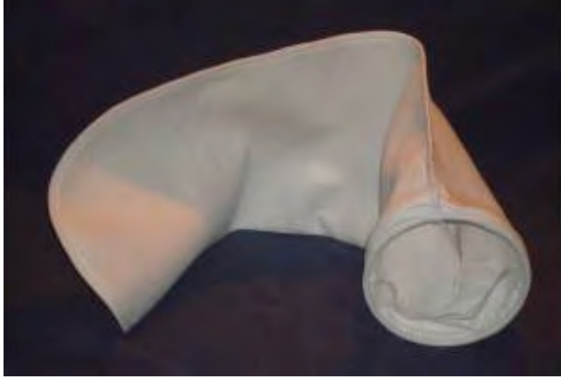
Figure 7. Filter bag that fits over the setting tank source of seawater.
