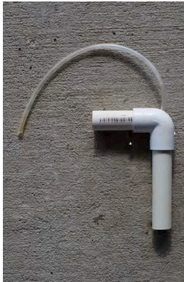
Figure 16. An airlift. 'L' shaped airlift with flexible air-hose and air-stone (top left). The air-hose is inserted into the airlift through a hole in the elbow and the air-stone attached to the hose (top right). The air-stone has to be pulled up into the airlift for water to be lifted (bottom).
