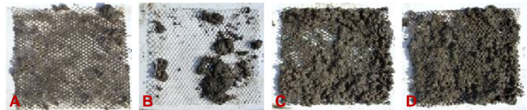
Figure 2. Net coating treatments (A, B, C, D) after three months deployment on a shellfish aquaculture lease.
