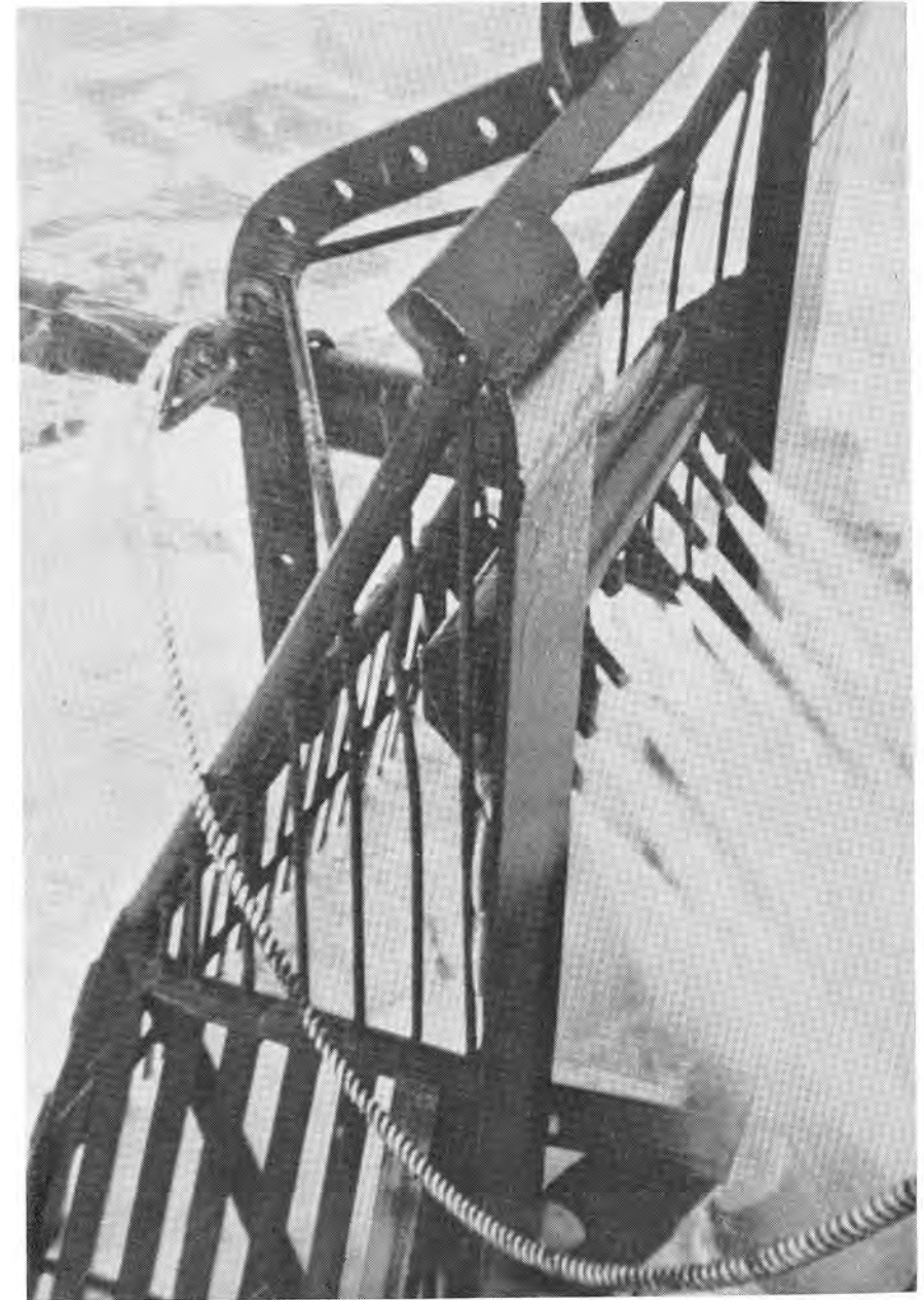
Figure 4. Nantucket dredge, showing manifold and water jets.
