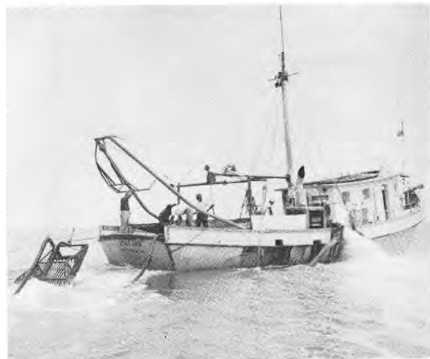
Figure 2. The modified shrimp trawler Little John , showing the "A" frame construction and the Nantucket dredge being lowered.
