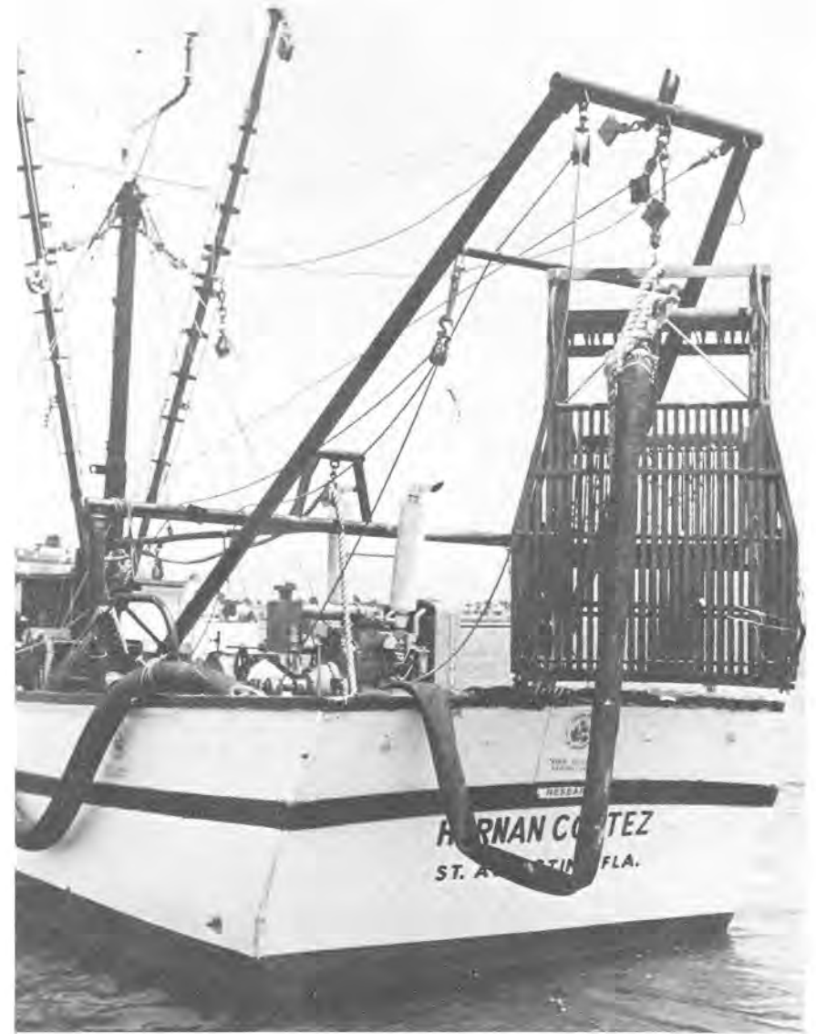
Figure 1. R/V Hernan Cortez and hydraulic Nantucket gear.
