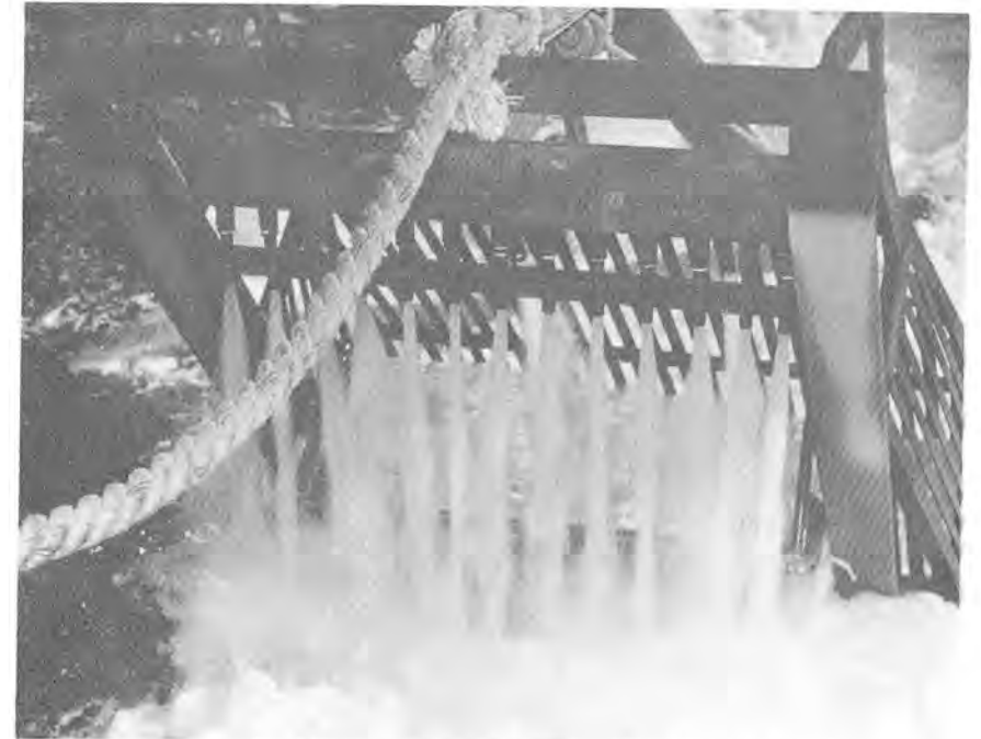
Figure 2. Water pressure used to force clams from substrate.
