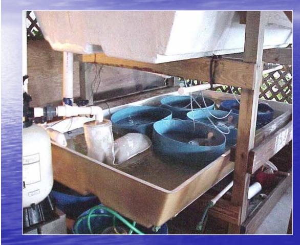
**Components:** – Fiberglass tank • 250 gallons Sand filter – Bag filters • 25 µm • 100 µm - Aeration Airlift pumps
