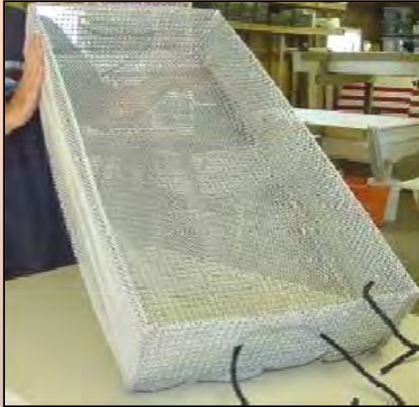
Bottom cages (3' x 1.5' x 6" deep) constructed of wire and lined with 4 mm polyester mesh material
