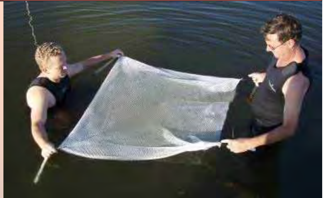
Bottom bags (4' x 4', 16 ft 2 ) made of 9 mm polyester mesh material
