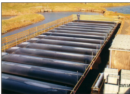
Figure 12. Outdoor culture of microalgae using polyethylene bags horizontally oriented to maximize illumination (courtesy Bay Shellfish, Tampa, FL).
