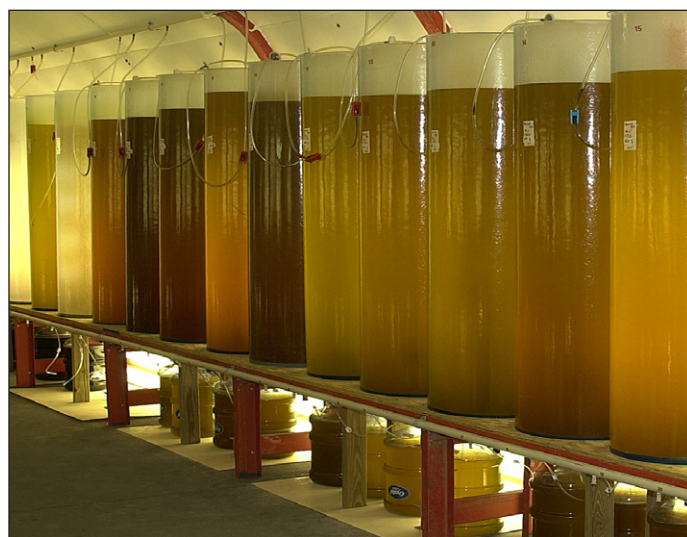
Figure 10. Translucent fiberglass cylinders (200-L) are commonly used for production of microalgae up to harvest and feeding. For large-scale algae production, they can be used to inoculate 2,000- to 5,000-L mass culture tanks.
