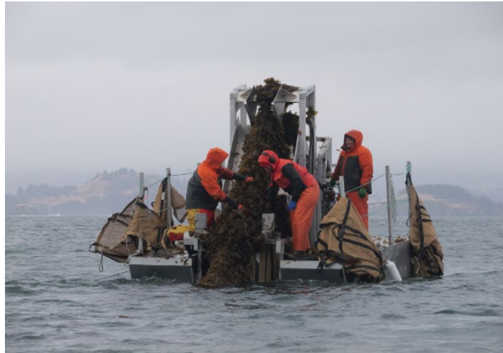
Figure 3.18: Specialized seaweed harvesting vessel built by Alf Pryor for Alaska Ocean Farms (Photo courtesy of James Currie, NOAA Alaska Regional Office)
