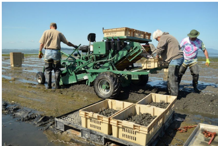
Figure 2.40: Manila clams in Samish Bay, Washington being harvested mechanically with a modified tulip bulb harvester (Photo courtesy of Bill Dewey, Taylor Shellfish Farm)
