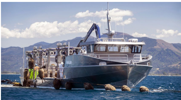
Figure 2.37: Harvesting vessel for a surface New Zealand style mussel longline farm with a davit crane system 88
