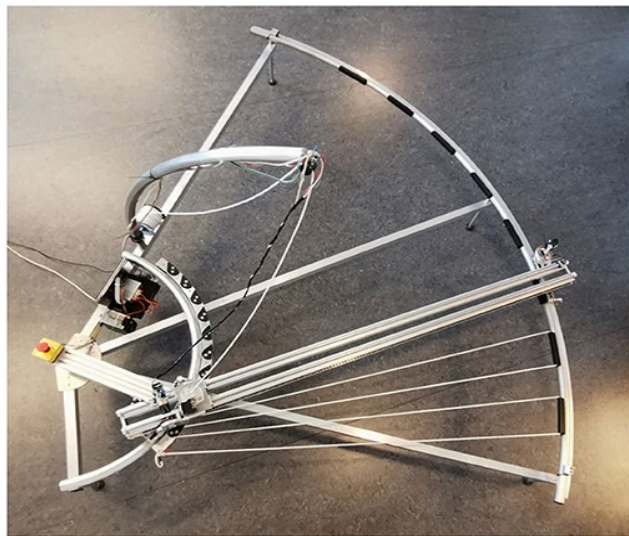
Figure 3.14: A prototype of only 90 degrees of the SPOKe macroalgae grow system 129
