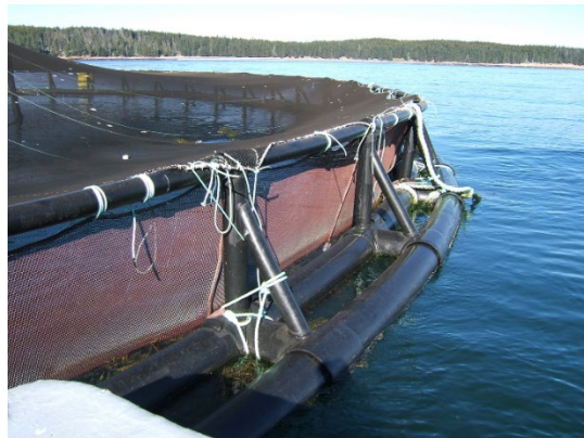
Figure 4.5: Floating net pen (Polar Cirkel™) (Photo courtesy of David Bean, NOAA Fisheries).
