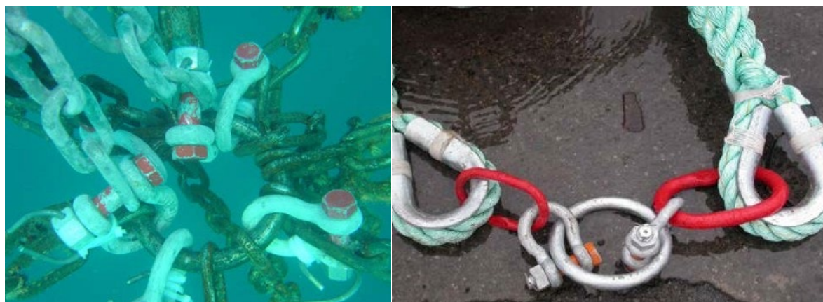
Figure 1.17: Round steel ring with multiple shackles connected (left) and connection of two open thimbles (with eye splice ropes) with round (silver) and oval (red) steel rings using a pair of shackles (right) 29
