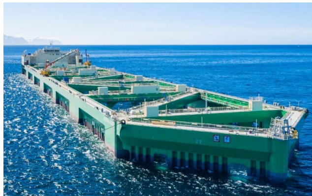
Figure 4.13: Havfarm floating rigid salmon aquaculture net pen in Norway 157
