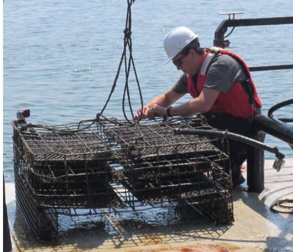
Figure 2.5: On-bottom six-compartment cage for up to 6 grow-out bags (Photo courtesy of Zachary Gordon, NOAA Fisheries)
