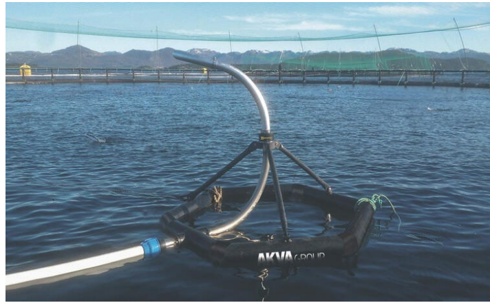
Figure 4.18: Airborne rotary feeder in the center of a fish net pen 165
