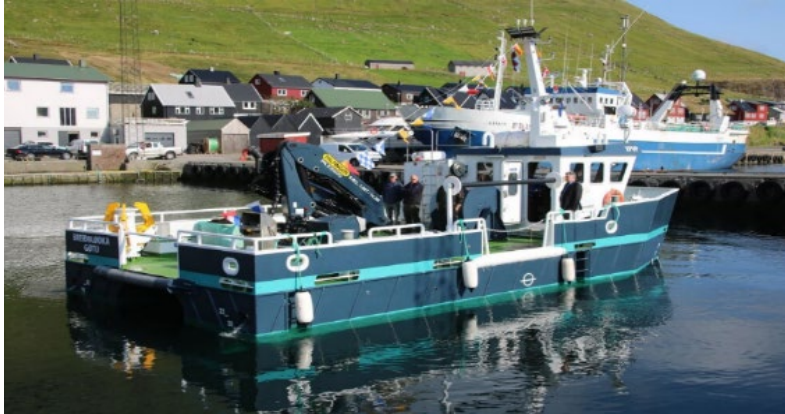
Figure 3.19: Specialized kelp harvesting vessel used by Ocean Rainforest 142
