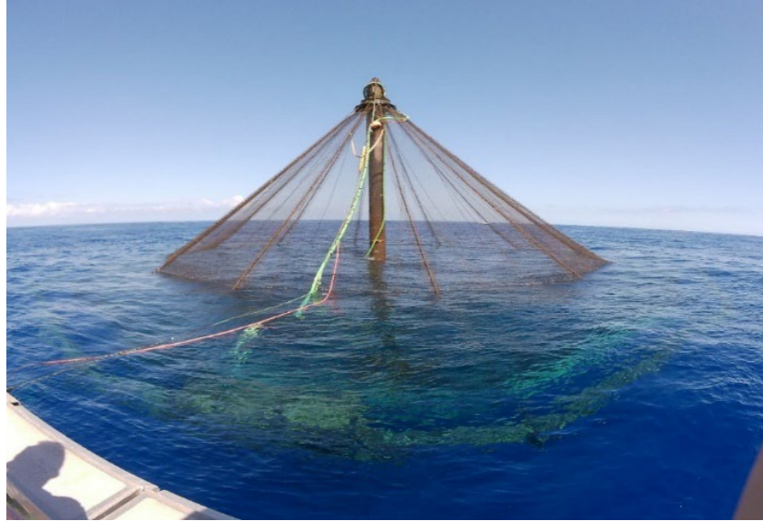
Figure 4.11: An Innovasea Sea Station™ cage raised to the surface at Blue Ocean Mariculture in Kona, Hawaii (Photo courtesy of Kirsten Jeong for NOAA Fisheries) 156
