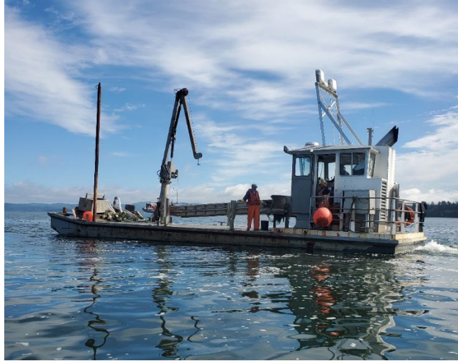
Figure 2.39: On-bottom oyster dredge in Washington (Photo courtesy of Bobbi Hudson, Pacific Shellfish Institute)
