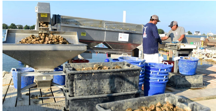
Figure 2.38: Oyster tumbler used to sort oysters by size and agitate the oysters to remove biofouling and smooth the shells for market 92
