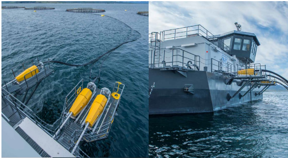
Figure 4.20: (Left) Feed Barge (with feed hoses deployed) and (Right) feed hoses from a feed barge extending out to fish net pens 167
