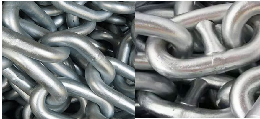
Figure 1.12: Studless (left) and Studded (right) chain links 23
