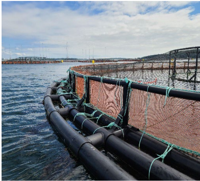
Figure 4.16: Three ring floating net pen with jump fence (reddish-brown) and avian predator netting attached (Photo courtesy of David Bean, NOAA Fisheries)
