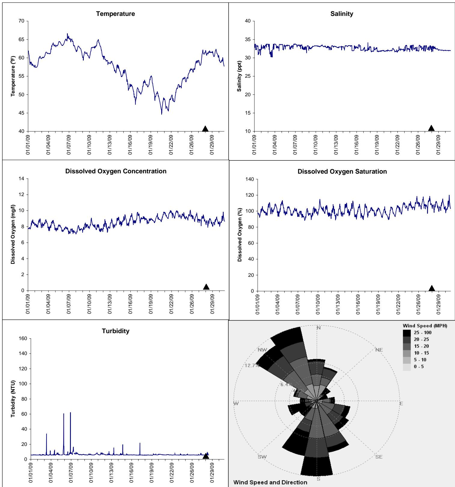
▲ Monitoring Equipment Exchanged (sonde deployment)
