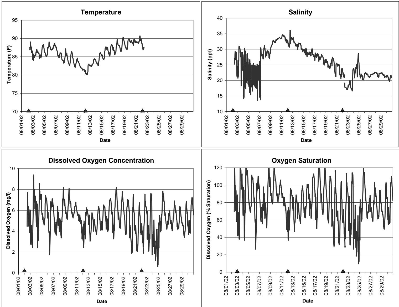
▲ Monitoring equipment exchanged (sonde deployment)
