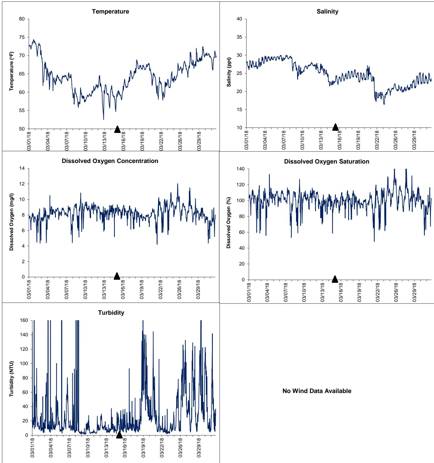
▲ Monitoring Equipment Exchanged (sonde deployment)
