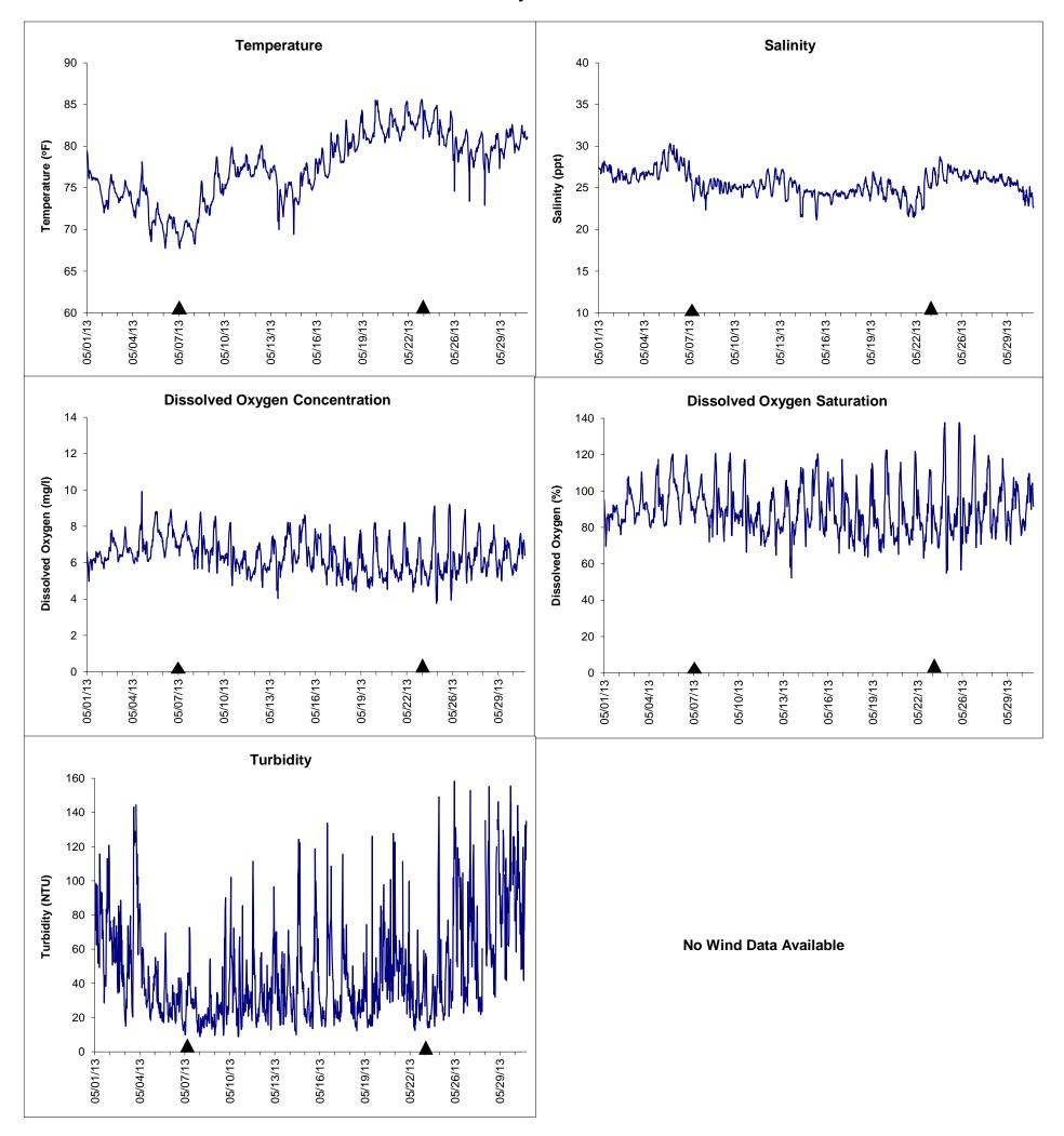
▲ Monitoring Equipment Exchanged (sonde deployment)
