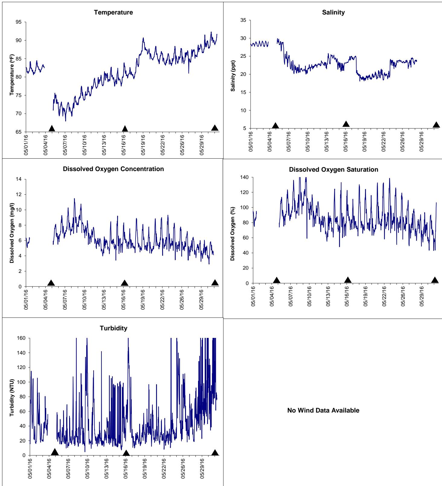
▲ Monitoring Equipment Exchanged (sonde deployment)
