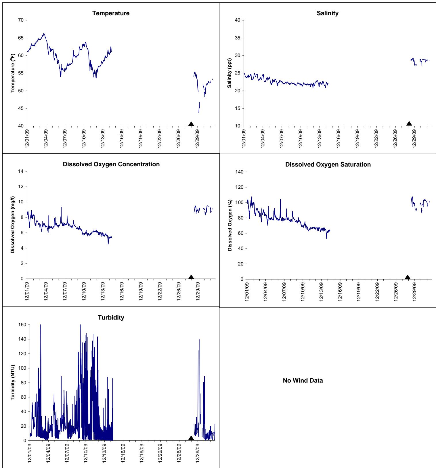
▲ Monitoring Equipment Exchanged (sonde deployment)
