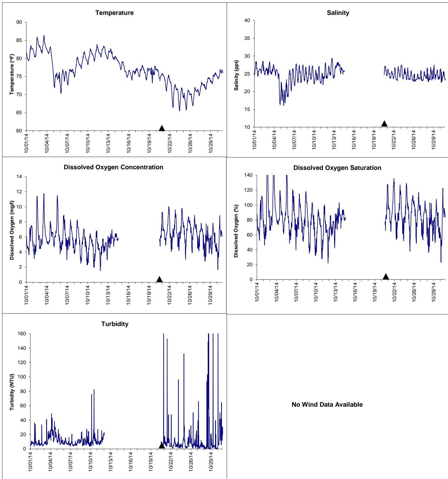
▲ Monitoring Equipment Exchanged (sonde deployment)
